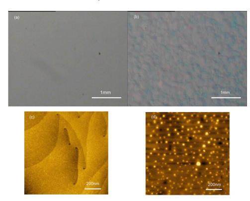
FIG. 3. (Color online) Nomarski optical microscope and  $1 \times 1 \mu m^2$  area AFM images of as-grown GaN surface for [(a) and (c)] sample A and [(b) and (d)] sample B.
