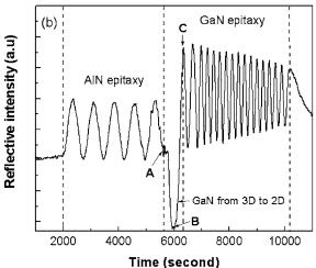
FIG. 4. Reflectivity monitored during semi-insulating GaN epitaxy on (a) LT-GaN nucleation and (b) AlN buffer. The 3D-2D transition is clearly visible in GaN grown on AlN buffer.
