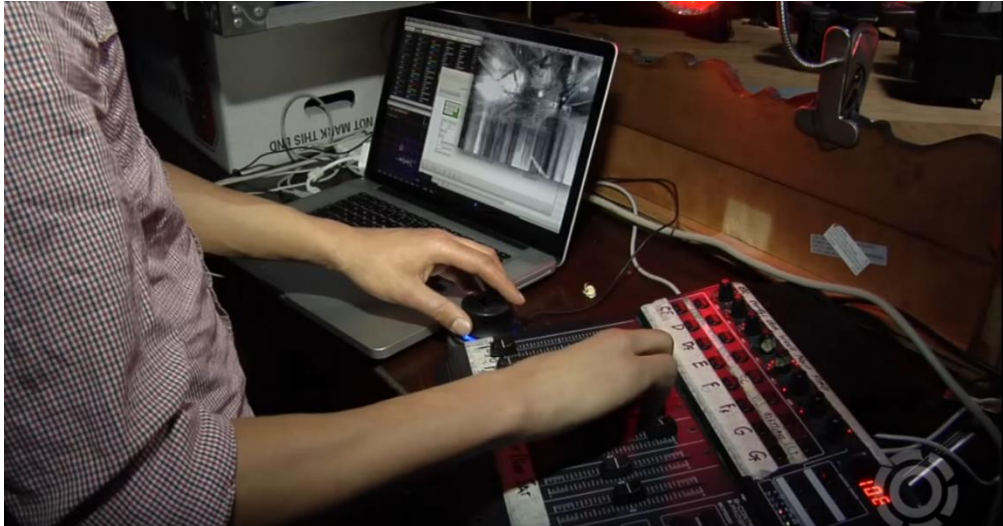
Fig. 45. “An Interview with Tarik Barri on Tour with Monolake”, Cycling ’74, Tarik Barri’s Input devices including 3D Space Navigator and Midi Controller.
