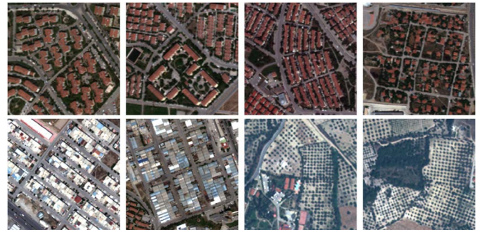
Fig. 1. Examples of compound structures in WorldView-2 images. Each 150 \times 150 pixel window includes one or more examples for residential, industrial, and agricultural structures composed of various spatial arrangements of primitives (buildings and trees) with different color and shape characteristics.
