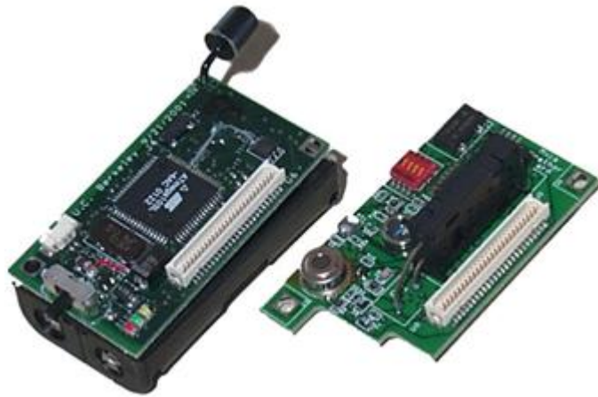
Figure 2.3: Mica Hardware Platform
