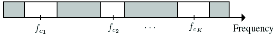
Fig. 1. Illustration of dispersed spectrum utilization in the cognitive radio system, where the white spaces represent the available bands.
