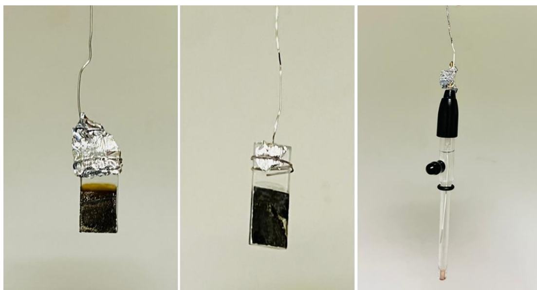
Fig 6. 2 Novel Experimental Setup for Conducting Overall Water-Splitting Experiments.
