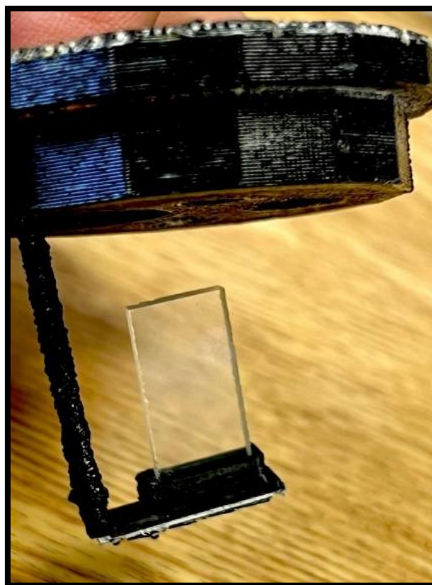
Fig 4. 1 Image of the 3D-printed stage for all the HER and OER reactions under magnetic field.
