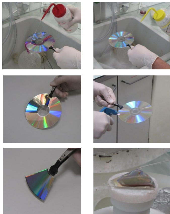
Figure 4.4: (a) Acetone treatment. (b) Isopropanol treatment. (c) Drying with dry nitrogen flow. (d) Dried disc. (e) Slice from the disc. (f) PMMA spin coating.
