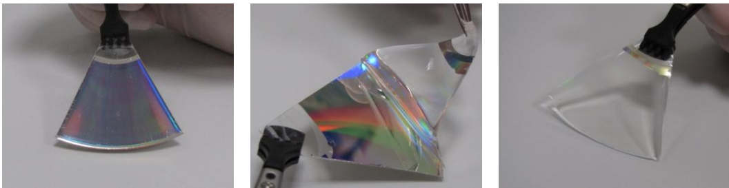
Figure 4.8: (a) PDMS molded disc. (b) Peeling off the PDMS mold. (c) PDMS mold having the replica of the pattern on the disc surface.
