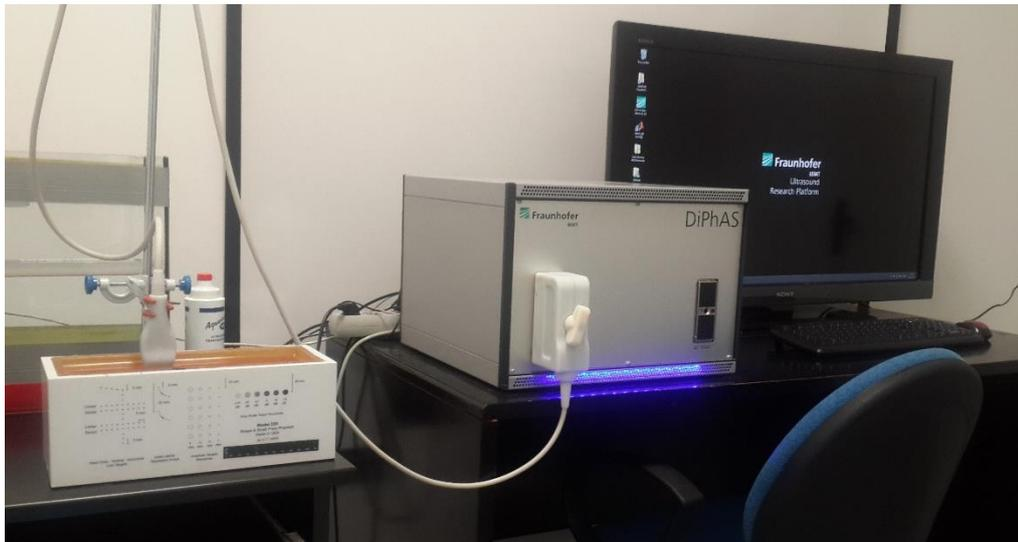
Figure 3.6: Experimental setup for phantom measurements. The setup consists of DiPhAS integrated with a personal computer, a phantom, a phased array transducer positioned on top of the phantom surface, and a holder for fixing the transducer array position.
