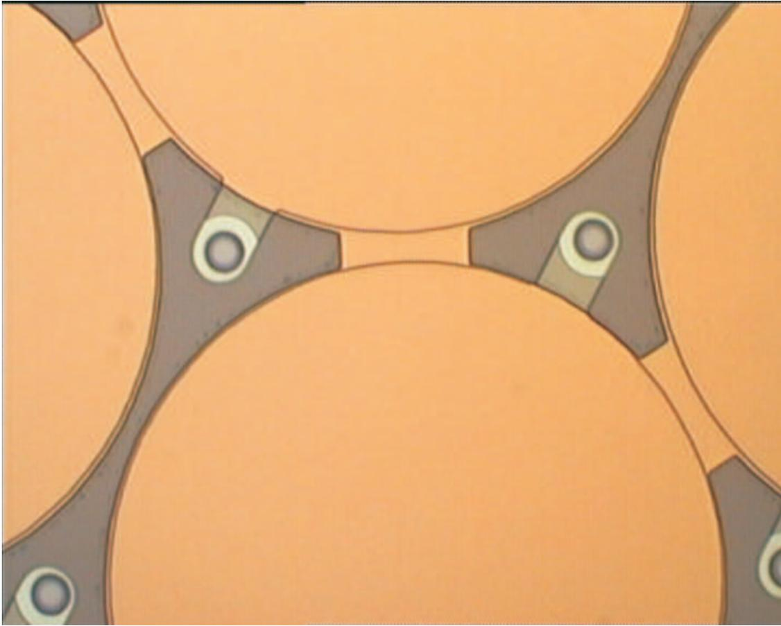
Figure 4.3: A micrograph of a CMUT cell during the release step. The CMUT cell in the micrograph has  $30 \mu\text{m}$  radius. Two smaller circles connected to the cell are the etch holes, where the chromium etchant enters the cavity during release step. Notice that etched and remaining parts of the chromium layer are clearly seen around the etch holes.
