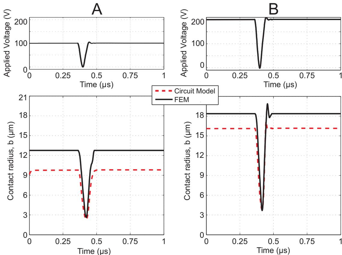
Figure 3.4: Variation of the contact radius,  $b$ , as calculated by FEM (solid) and equivalent circuit simulation (dashed) as a function of time, when a CMUT is excited by negative 100 V (A) and 200 V (B) pulses on a bias with equal amplitude. The applied signals are depicted at the top. The simulated CMUT has a silicon nitride membrane with  $a=30 \mu\text{m}$ ,  $t_m=1.4 \mu\text{m}$ ,  $t_i=0.4 \mu\text{m}$ ,  $t_g=0.2 \mu\text{m}$ .
