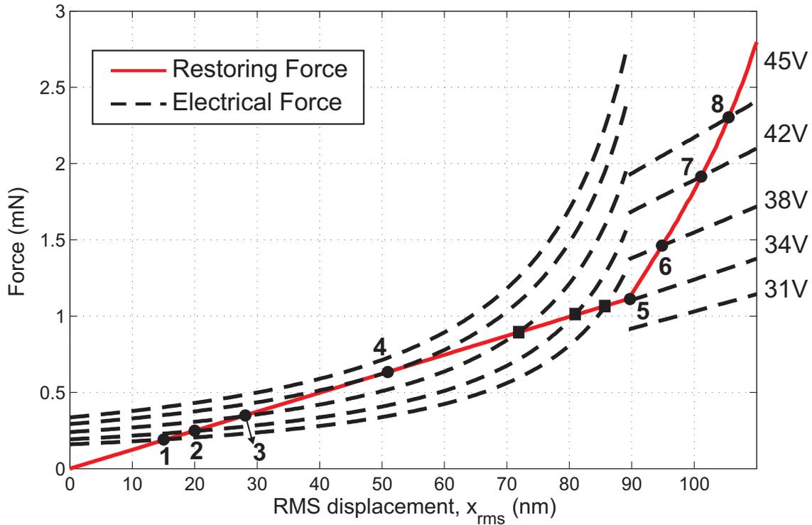
Figure 2.8: The electrostatic attraction and mechanical restoring forces of a silicon nitride membrane with  $a=30 \mu\text{m}$ ,  $t_m=1.5 \mu\text{m}$ ,  $t_i=0.2 \mu\text{m}$ ,  $t_g=0.2 \mu\text{m}$  for different values of DC bias as a function of  $x_{rms}$ . The atmospheric pressure is neglected.
