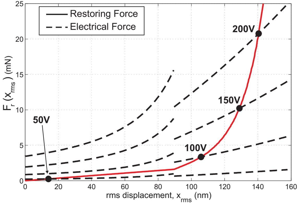
Figure 2.6: Mechanical restoring force (solid) and electrostatic attraction forces (dashed) when the bias is 50, 100, 150 and 200 Volts as a function of  $x_{rms}$ . The dimensions of silicon nitride membrane:  $a=25 \mu\text{m}$ ,  $t_m=1.5 \mu\text{m}$  and  $t_i=0.4 \mu\text{m}$  and  $t_g=0.2 \mu\text{m}$ . The intersection point of the curves is the static equilibrium position, when the atmospheric pressure is neglected.
