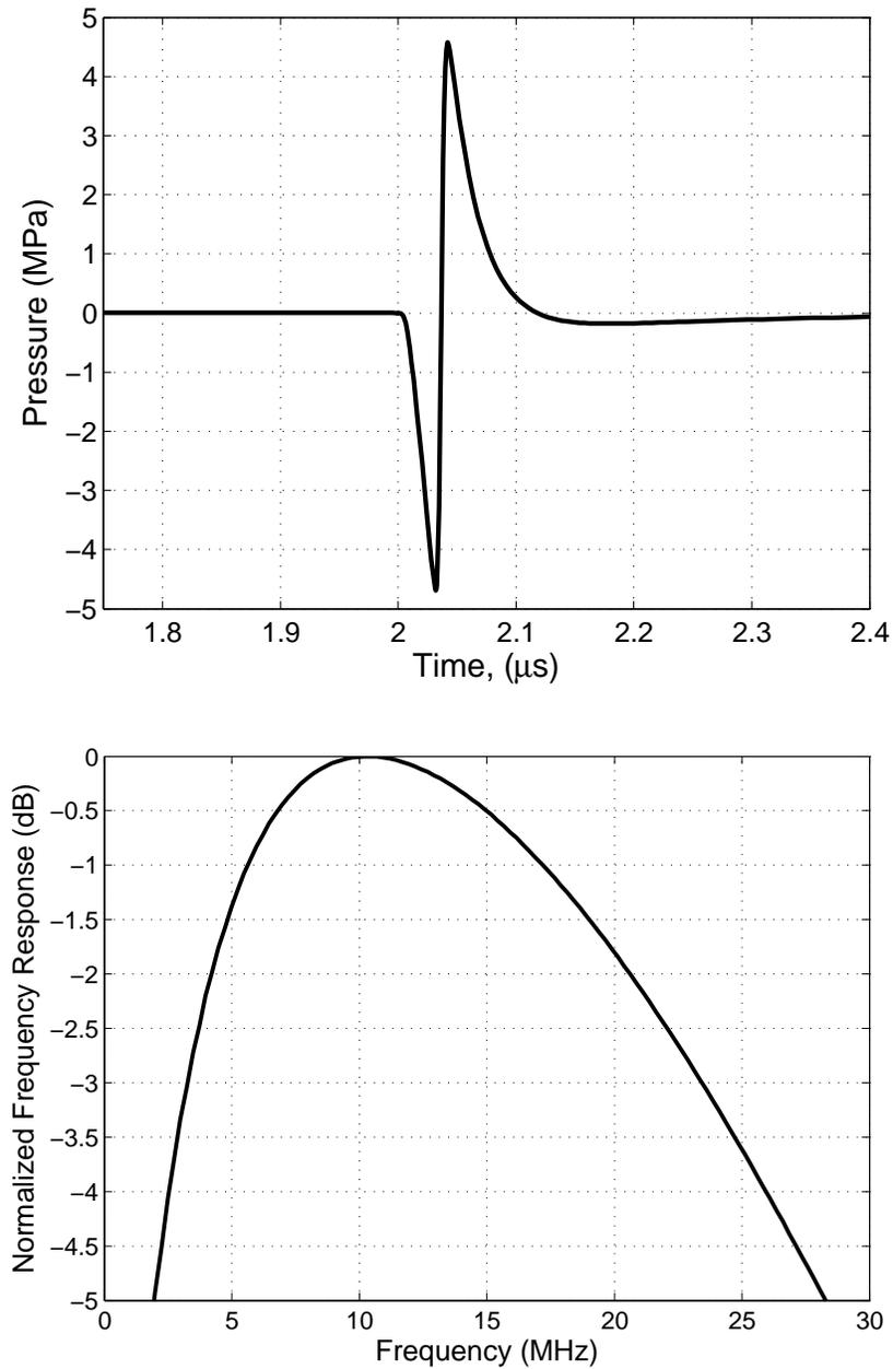
Figure 5.19: Simulated acoustic pulse (top) and its spectrum (bottom) by the designed CMUT with dimensions:  $a = 81\mu\text{m}$ ,  $t_m = 5\mu\text{m}$ ,  $t_g = 0.1\mu\text{m}$ ,  $t_i = 0.2\mu\text{m}$ . The electrical excitation is a 100V pulse with 22 ns pulse width; and 10ns rise and fall times.
