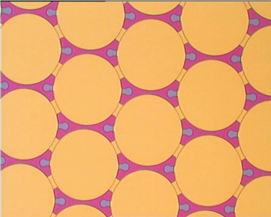
Figure 4.2: A micrograph of a CMUT cell during fabrication after top electrode deposition. The CMUT cell in the micrograph has  $40 \mu\text{m}$  radius. Two smaller circles connected to the cell are the regions for the etch holes, where the chromium etchant enters the cavity during release step.
