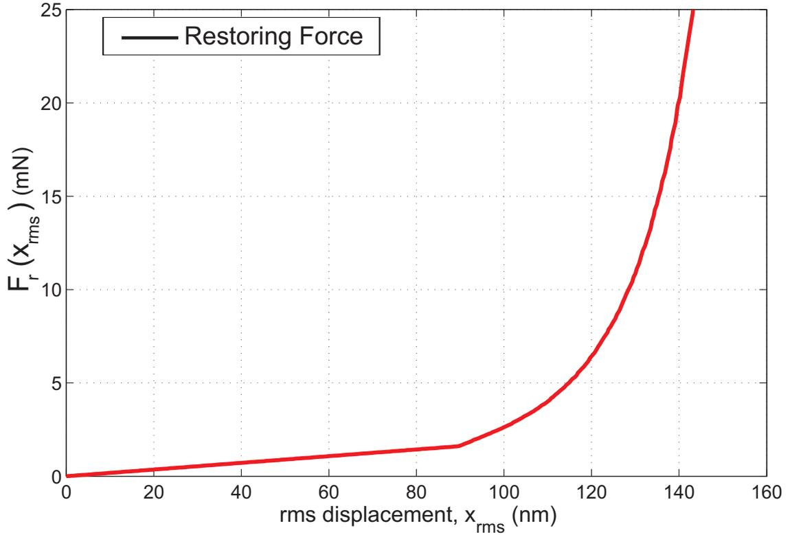
Figure 2.5: Mechanical restoring force (solid) as a function of  $x_{rms}$ . The dimensions of silicon nitride membrane:  $a=25 \mu\text{m}$ ,  $t_m=1.5 \mu\text{m}$ ,  $t_i=0.4 \mu\text{m}$  and  $t_g=0.2 \mu\text{m}$ .
