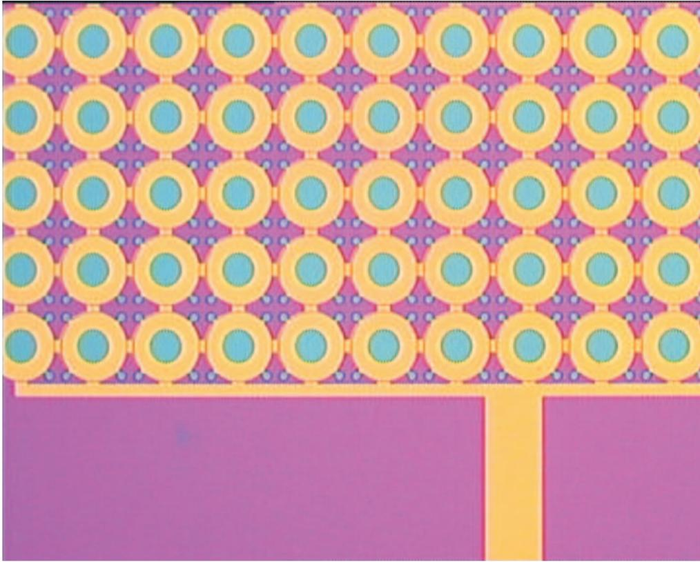
Figure 5.6: An optical micrograph of a fabricated CMUT array. The ring shaped top electrode has 50% inner radius. at 121 cells (11 by 11) each with a radius of  $a=30 \mu\text{m}$  and a cell to cell separation of  $5 \mu\text{m}$ . The aperture size is  $0.71 \text{ mm}$  by  $0.71 \text{ mm}$  and the fill factor is 67%.
