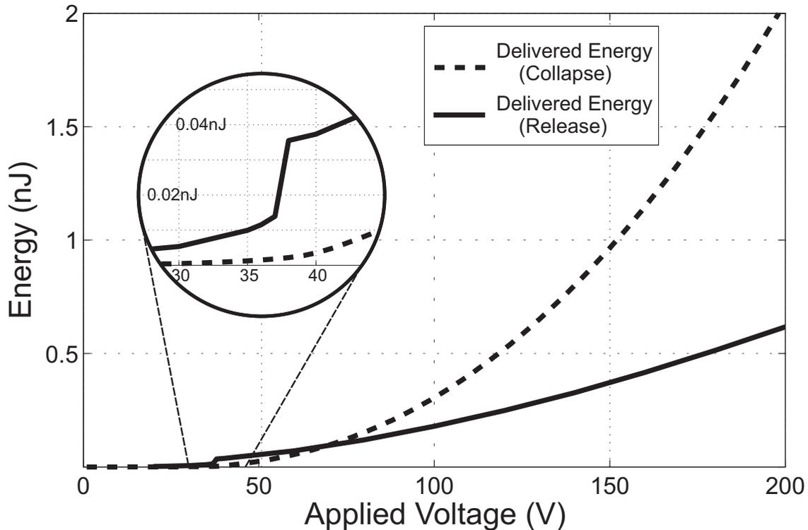
Figure 5.2: Delivered energy during the release (solid) and collapse (dashed) parts of a unipolar pulse cycle. CMUT parameters:  $a = 30\mu\text{m}$ ,  $t_m = 1.4\mu\text{m}$ ,  $t_g = 0.2\mu\text{m}$ ,  $t_i = 0.4\mu\text{m}$ .
