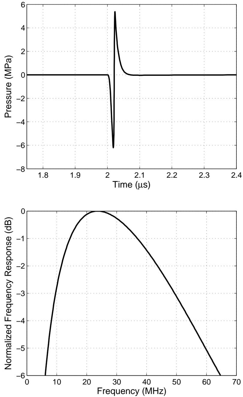
Figure 5.20: Simulated acoustic pulse (top) and its spectrum (bottom) by the designed CMUT with dimensions:  $a = 42\mu\text{m}$ ,  $t_m = 2.3\mu\text{m}$ ,  $t_g = 70\text{nm}$ ,  $t_i = 0.2\mu\text{m}$ . The electrical excitation is a 100V pulse with 10 ns pulse width; and 10ns rise and fall times.
