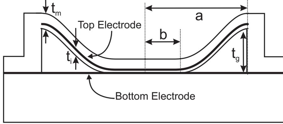
Figure 2.2: Cross sectional view of a collapsed clamped circular membrane with radius  $a$ , thickness  $t_m$  and gap height of  $t_g$ . The top electrode is at a distance  $t_i$  above from the gap.  $b$  is the contact radius. The bottom electrode is assumed to be at the top of the substrate.
