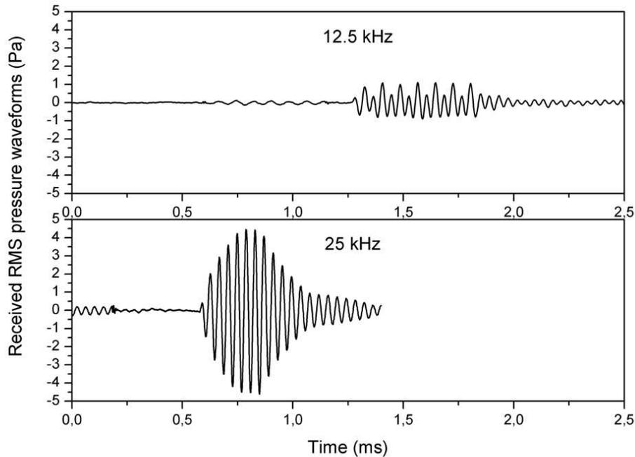
Figure 6.6: Recorded pressure waveforms for the cell B for 100V peak-to-peak sinusoidal burst excitation at 12.5 kHz and 25 kHz on 50V DC bias.
