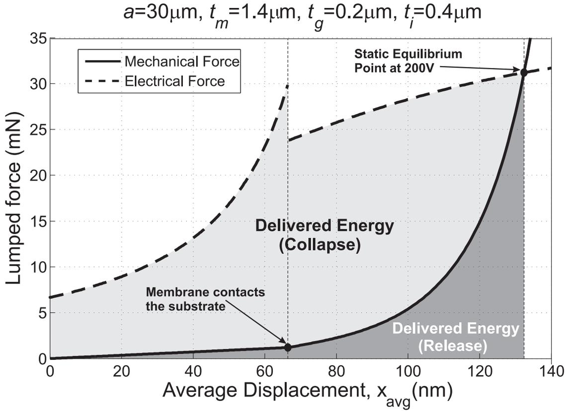
Figure 5.1: The electrical attraction force (dashed) at a bias of 200 V and the mechanical restoring force (solid) as a function of average displacement,  $x_{avg}$ . The membrane has a radius of  $30 \mu\text{m}$  and a thickness of  $1.4 \mu\text{m}$ . The buried electrode covering the full surface is  $0.4 \mu\text{m}$  away from  $0.2 \mu\text{m}$  thick gap.
