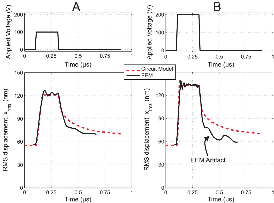
Figure 3.6: Variation of  $x_{rms}$  as calculated by FEM (solid) and equivalent circuit simulation (dashed) as a function of time, when the CMUT is excited by 10 ns rise or fall time pulses with 100 V (A) and 200 V (B) amplitudes. The simulated CMUT has a silicon nitride membrane with  $a=30 \mu\text{m}$ ,  $t_m=2 \mu\text{m}$ ,  $t_i=0.4 \mu\text{m}$ ,  $t_g=0.16 \mu\text{m}$  resulting in a collapsed state under atmospheric pressure.
