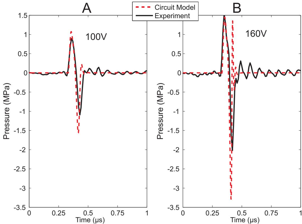
Figure 3.8: Comparison of the equivalent circuit simulations (dashed) to experimental results (solid). The CMUTs used in the experiments have  $a=30\ \mu\text{m}$ ,  $t_m=1.4\ \mu\text{m}$ ,  $t_g=0.2\ \mu\text{m}$  and  $t_i=0.4\ \mu\text{m}$ . They are excited with signals of 120 and 160V negative amplitudes on equal amplitude DC biases.
