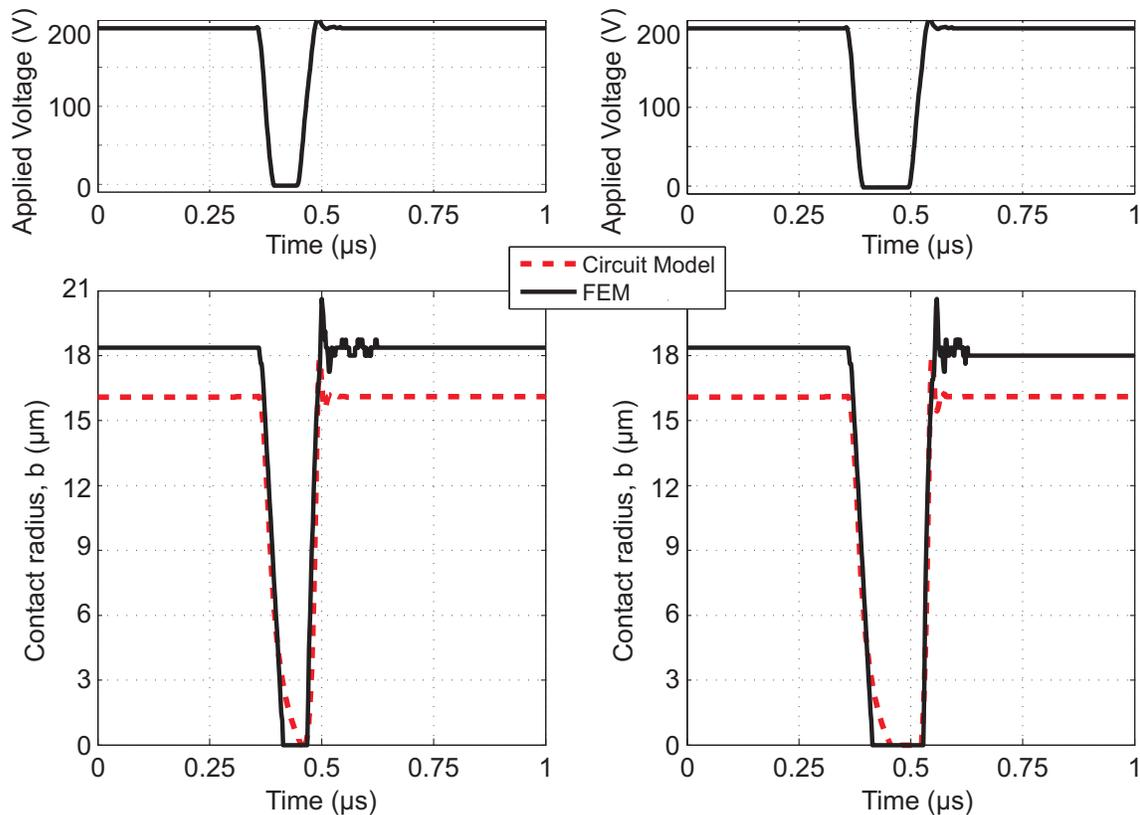
Figure 3.5: Variation of the contact radius,  $b$ , as calculated by FEM (solid) and equivalent circuit simulation (dashed) as a function of time, when a CMUT is excited by 200 Volts pulses with different widths on a bias with equal amplitude. The applied signals are depicted at the top. The simulated CMUT has a silicon nitride membrane with  $a=30 \mu\text{m}$ ,  $t_m=1.4 \mu\text{m}$ ,  $t_i=0.4 \mu\text{m}$ ,  $t_g=0.2 \mu\text{m}$ .
