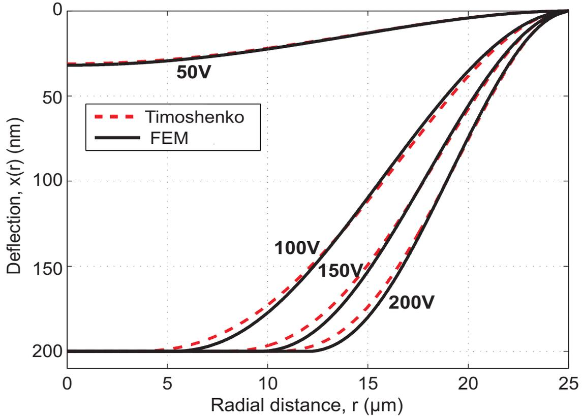
Figure 2.7: Displacement profiles calculated by electrostatic FEM simulations (solid) and by Timoshenko's plate deflection under uniform pressure (dashed) for a silicon nitride membrane with  $a=25 \mu\text{m}$ ,  $t_m=1.5 \mu\text{m}$ ,  $t_i=0.4 \mu\text{m}$ ,  $t_g=0.2 \mu\text{m}$  for different values of bias. The atmospheric pressure is neglected.
