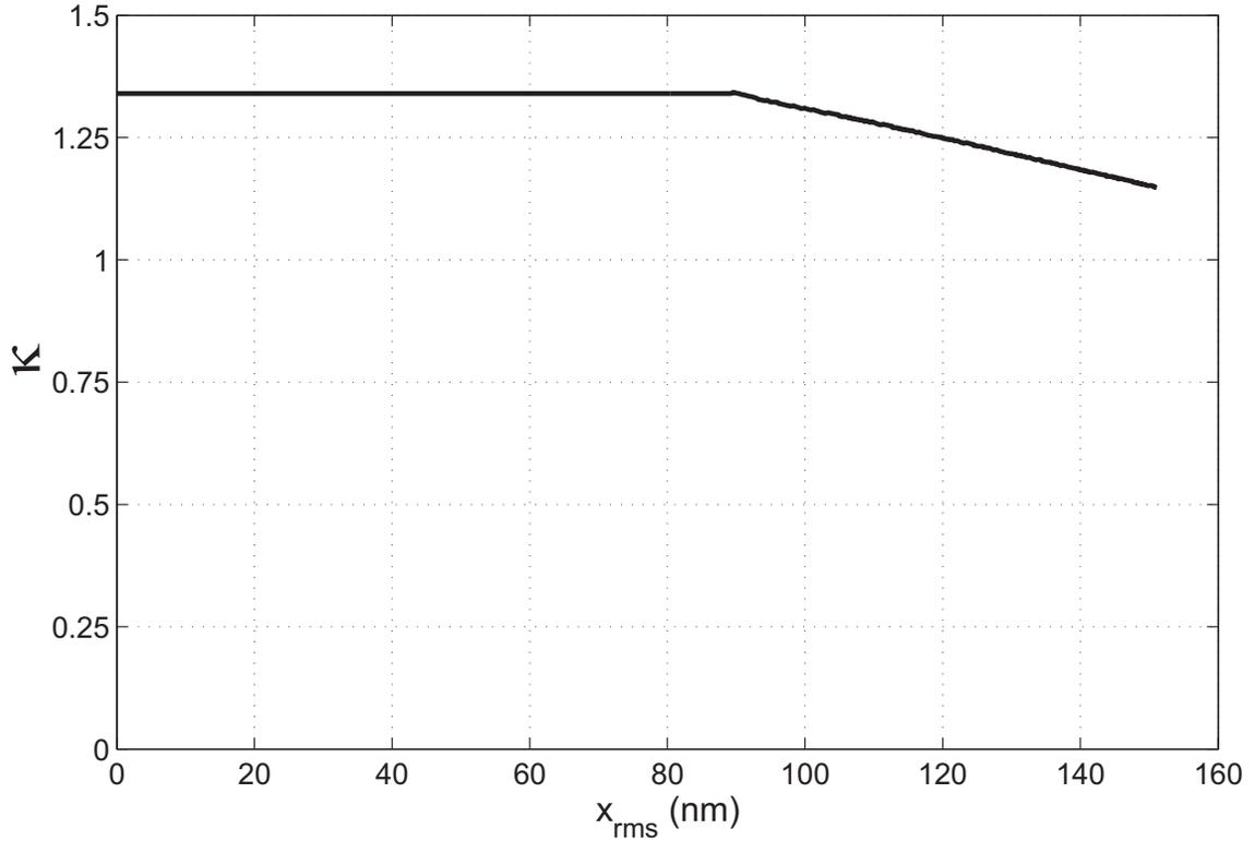
Figure 2.4: The correction factor,  $\kappa$  as a function of rms displacement for a CMUT membrane with dimensions:  $a=25 \mu\text{m}$ ,  $t_m=1.5 \mu\text{m}$ ,  $t_i=0.4 \mu\text{m}$  and  $t_g=0.2 \mu\text{m}$ . For this figure,  $\gamma_0$  of equation (2.4) is 3.16.
