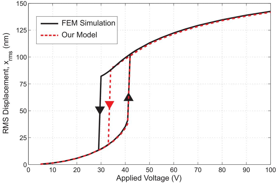
Figure 2.9: RMS displacement of a silicon nitride membrane with  $a=30 \mu\text{m}$ ,  $t_m=1.5 \mu\text{m}$ ,  $t_i=0.2 \mu\text{m}$ ,  $t_g=0.2 \mu\text{m}$  as a function of applied voltage. The displacements calculated by our method (dashed) are compared to FEM simulation results (solid). The effect of the atmospheric pressure is neglected.
