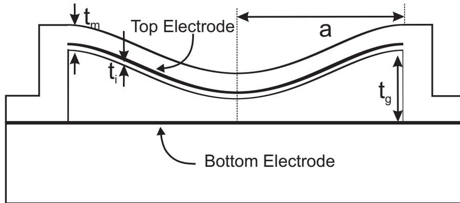
Figure 2.1: Cross sectional view of an uncollapsed clamped circular membrane with radius  $a$ , thickness  $t_m$  and gap height of  $t_g$ . The top electrode is at a distance  $t_i$  above from the gap. The bottom electrode is assumed to be at the top of the substrate.
