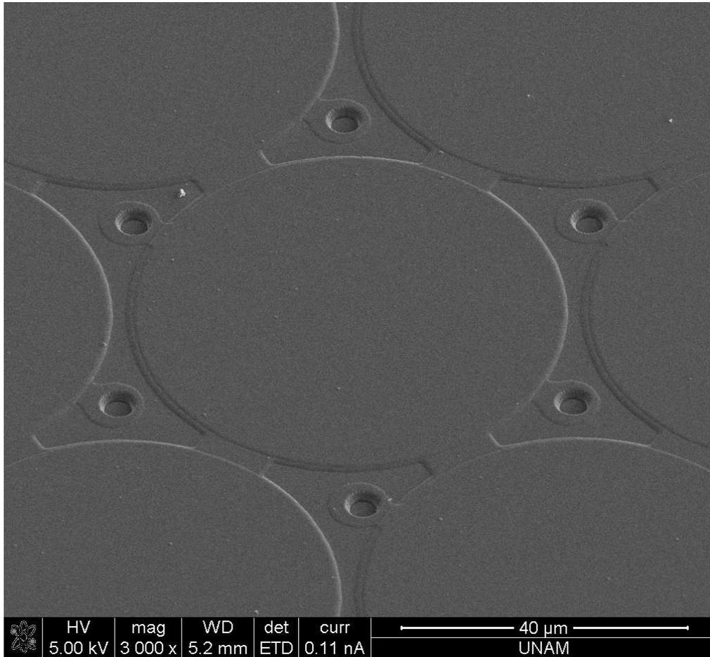
Figure 4.6: A SEM image of a fabricated CMUT array with full electrode coverage top electrodes. Sealed etch holes are seen at the corners of a CMUT cell.
