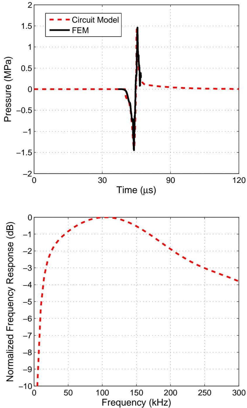
Figure 6.9: Transient FEM and equivalent circuit simulations for the acoustic pulse (top) and its spectrum (bottom) generated by the designed CMUT with dimensions:  $a=1.4\text{mm}$ ,  $t_m=75\mu\text{m}$ ,  $t_g=3\mu\text{m}$ ,  $t_i=1\mu\text{m}$ . The electrical excitation is a 500V pulse with  $4.8\mu\text{s}$  pulse width.
