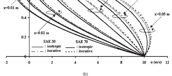
**Figure 9** Comparison of isotropic and iterative methods by lubricant (a) mass flow rate and (b) longitudinal (y-) velocity profiles.
