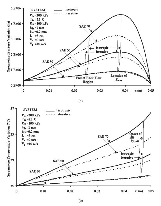
**Figure 10** Comparison of isotropic and iterative methods by lubricant (a) pressure and (b) temperature.
