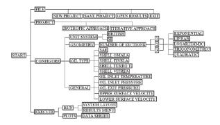
Figure 2 Hierarchical structure of "HYDRO-LUB."
