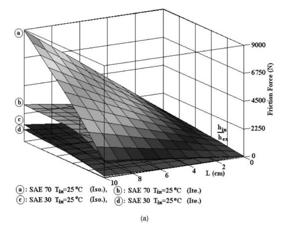
**Figure 11** Comparison of isotropic and iterative methods by (a) friction force and (b) load for different bearing lengths and inlet-exit height ratios.
