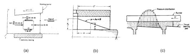
Figure 1 (a): Pressure and shear forces acting on the infinitesimal oil element, (b)-(c) linear and second order oil-pressure distribution on simple bearing geometries [13].
