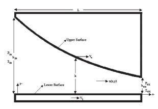
Figure 8 Schematic layout of slider bearing with curved upper surface.
