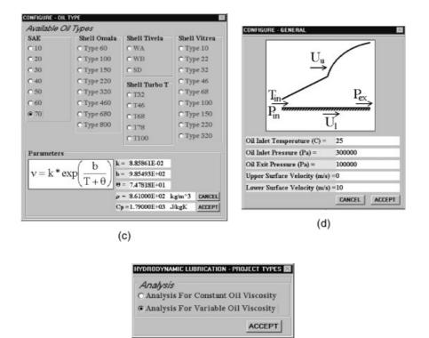
**Figure 4** Configuration menus of "HYDRO-LUB" (a) Unit system, (b) Geometry, (c) Oil type, (d) General, (e) Project type.
