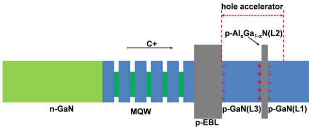
FIG. 1. Schematic energy band diagram for the InGaN/GaN LED device with a hole accelerator (layer thickness not in scale), along with which we also show the polarization induced sheet charges at L1/L2, L2/L3, and p-EBL/L3 interfaces, respectively.
