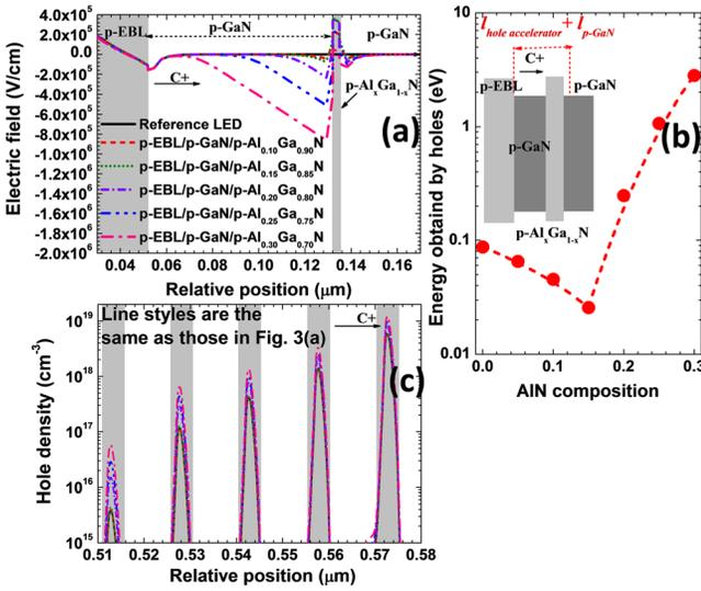
FIG. 3. (a) Electric field profiles, (b) kinetic energy obtained by holes, and (c) hole density profiles in the MQW region for the investigated LED devices with various AlN compositions in the p-Al<sub>x</sub>Ga<sub>1-x</sub>N (L2) layer. Data collected at 86 A/cm<sup>2</sup>.
