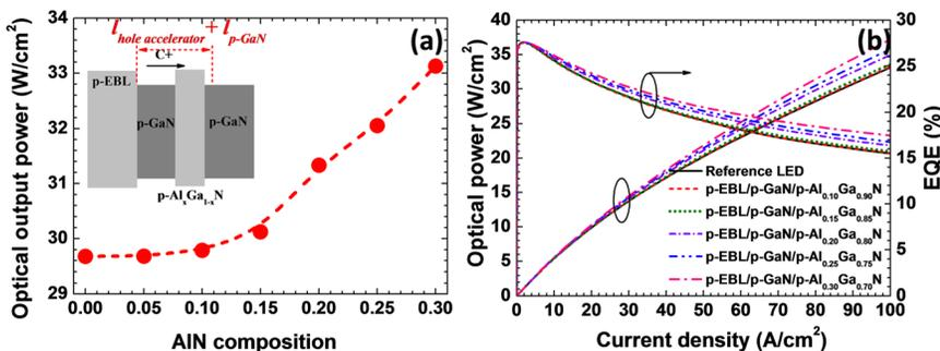
FIG. 4. (a) Optical output power in terms of different AlN alloys in the p-Al<sub>x</sub>Ga<sub>1-x</sub>N (L2) layer at the current density level of 86 A/cm<sup>2</sup> and (b) optical output power and EQE as a function of the injection current density for all the studied LED devices.
