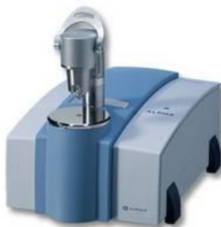
Figure 4.6 Bruker ALPHA Platinum ATR single reflection diamond based ATR spectrometer that was used in this study. Taken from ref #72.
