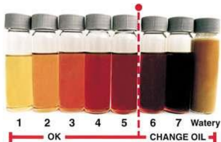
Figure 3.10 Color changes of lubricating oil during degradation (oxidation) [66].
