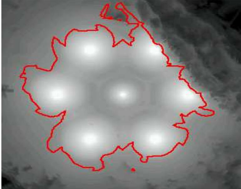
Fig. 7. 95 percent coverage probability contour for a 7-station DVB-T cell structure. The center station is at N 38° 30' 00", E 33° 30' 00". The stations are separated by 27 km., and the central station radiates 100 W, the remaining six stations on the edge of the cell radiate 1 kW each. Frequency is 826 MHz.
