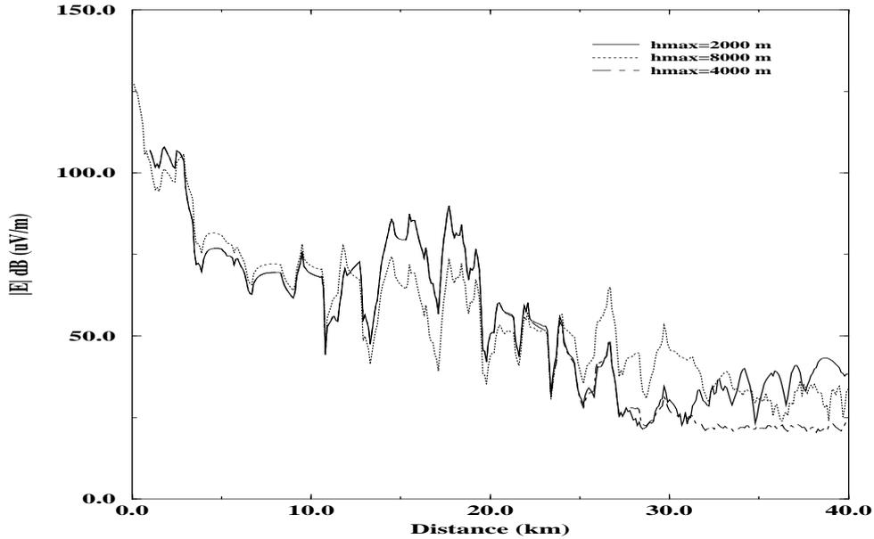
Fig. 5. Comparison of PWE solutions for different computation window heights.
