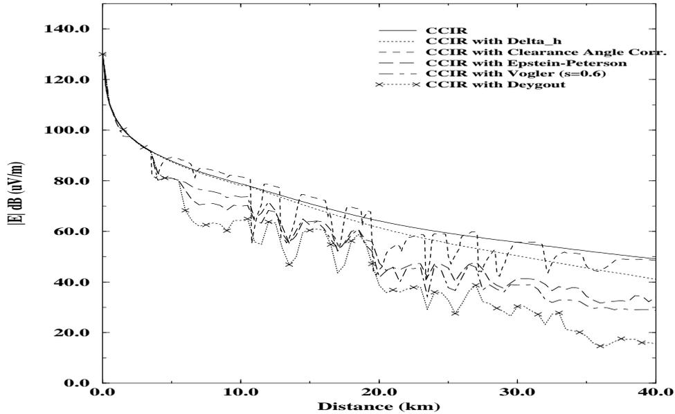
Fig. 2. Comparison of the field strengths predicted by different corrections to CCIR.
