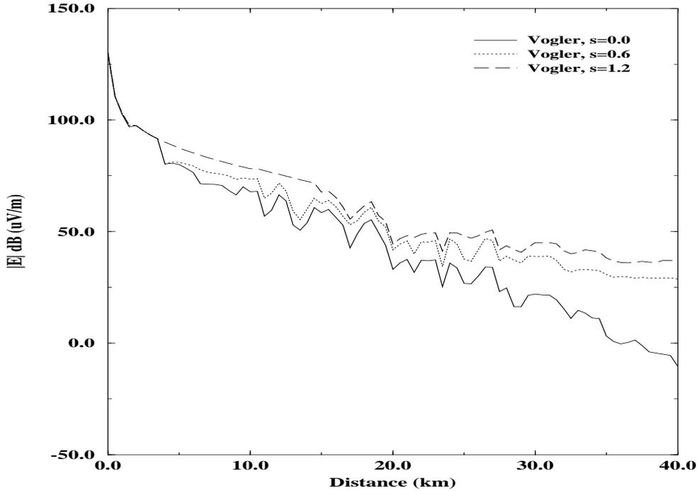
Fig. 3. Comparison of the field strengths predicted by the Vogler method with different selection parameter  $s$ .
