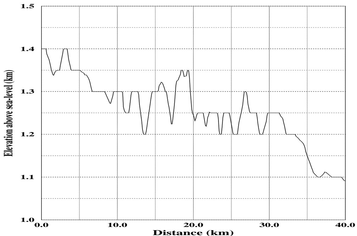
Fig. 1. Terrain profile above sea-level from TX-site 'A' (N 39° 30' 30", E 32° 37' 45") in the 180° azimuthal direction.
