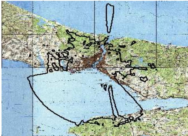
Fig. 6. 70 dB (uV/m) coverage contour of Çamlıca, Istanbul (N 41° 01' 40", E 29° 04' 08") analog TV station at UHF band with 40 dBW effective radiated power.
