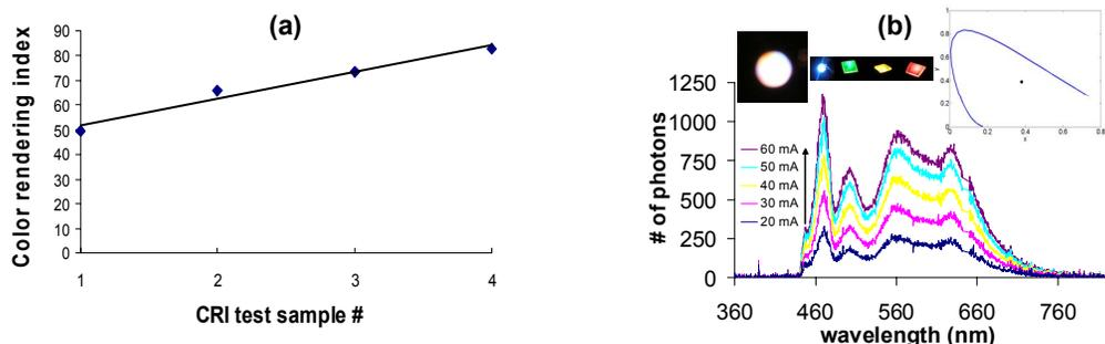
**Figure 2.** (a) Tuning color rendering index from Sample 1 to 4 by controlling the layer-by-layer assembly of polyfluorene and NC emitters and (b) emission spectra of blue polyfluorene and yellow-green-red CdSe/ZnS core-shell nanocrystals layer-by-layer hybridized on an n-UV InGaN/GaN LED at different levels of current injection at room temperature along with the pictures of generated lights and location of the corresponding operating  $(x, y)$  coordinates.
