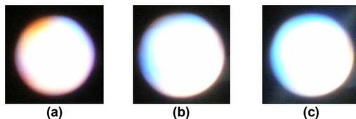
**Figure 1.** Images of white light emission from electrically driven nanocrystal-conjugated polymer hybridized WLEDs incorporating: (a) yellow NCs on blue polyfluorene, (b) yellow-green NCs on blue polyfluorene, and (c) yellow-green-red NCs on blue polyfluorene, all hybridized on n-UV LEDs.
