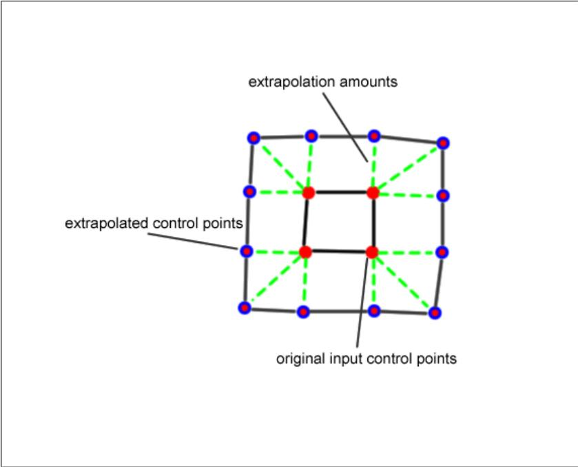
Figure 3.4: Extrapolation of additional control points from the original control points.
