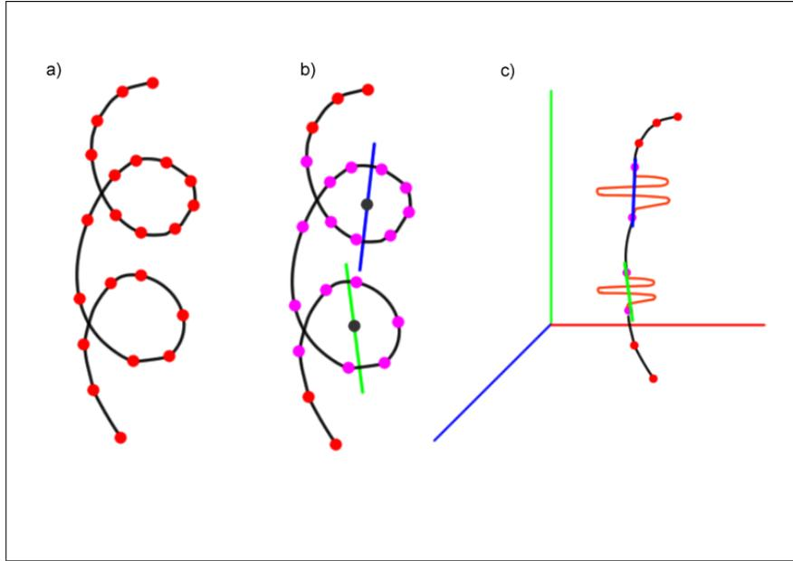
Figure 5.2: The process to solve a) ill defined skeleton strand sketches; b) the loops, loop directions and loop focal points are detected, c) by placing axis of rotation to focal points, the control points forming the loops are mapped to helical structures.
