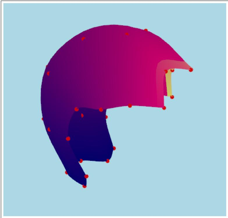
Figure 3.6: The color values are mapped to the u-v values of the patch.
