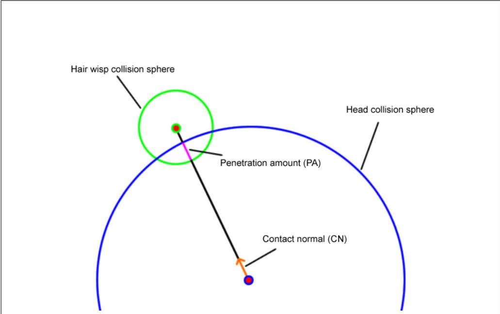
Figure 4.5: Wisp and head collision spheres and extracted collision information.
