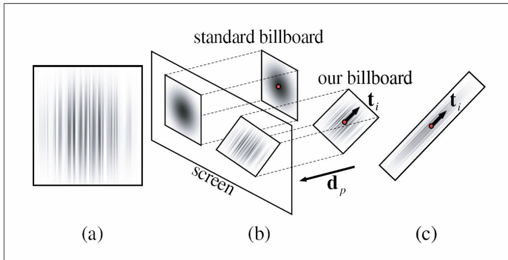
Figure 2.1: Bando et al.'s rendering technique. a) The alpha map applied to the textures, b,c) The alpha map applied to the hair texture is translated to the hair particle location and scaled in the hair direction.
