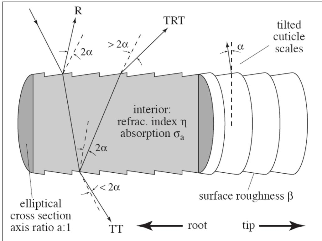
Figure 2.2: The hair fiber model used by Marschner.
