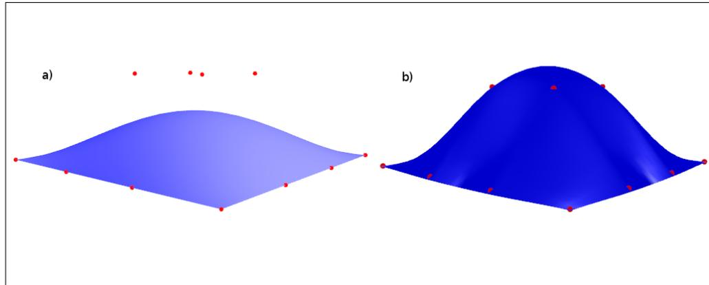
Figure 3.3: The difference between a) a Bezier patch and b) a Catmull-Rom patch with same control points.
