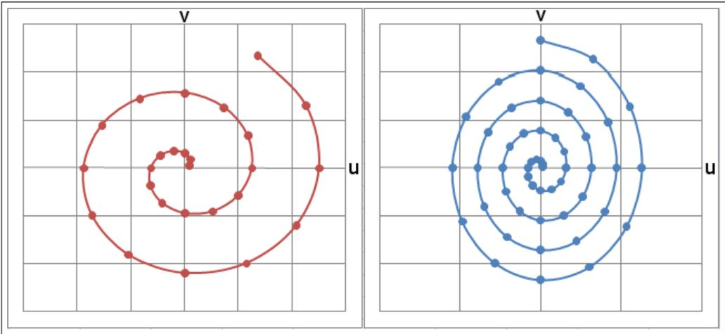
Figure 5.4: The Archimedes' spiral on the Catmull-Rom patch  $u$ - $v$  space. The points are obtained with 30 degree increments. The left hand spiral's closeness parameter  $c_{i,j}$  is greater than the right hand spiral's closeness parameter.
