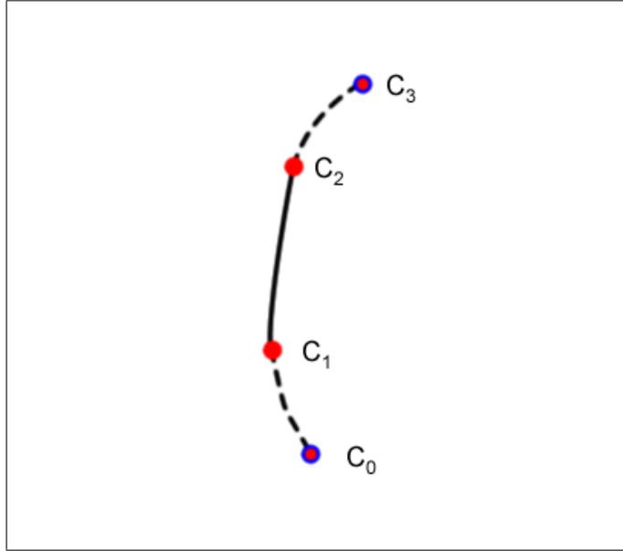
Figure 6.1: With the given control points  $C_0, C_1, C_2, C_3$ , a spline from  $C_1$  to  $C_2$  is obtained.
