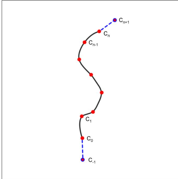
Figure 6.2: The extrapolation process of the additional Catmull-Rom spline control points.
