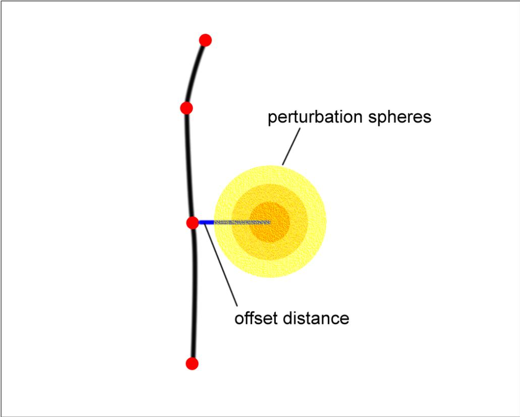
Figure 5.5: The blue vector represents the offset distance for that control point. According to the fuzziness parameter, the corresponding control point of the imitator strand is perturbed by randomly replacing it in the volumes defined by perturbation spheres. As fuzziness increases, the control point is randomized in a bigger perturbation sphere.
