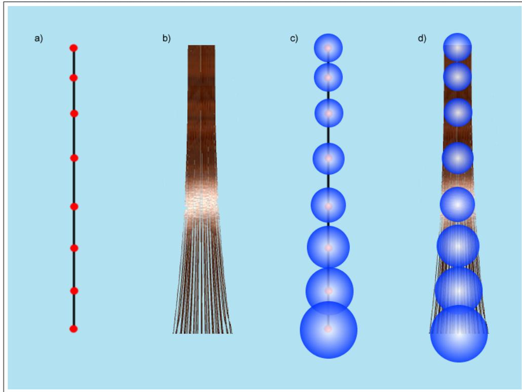
Figure 4.4: a) A skeleton strand that has increasing wisp closeness style parameter, b) the resultant wisp, c) wisp collision spheres located at skeleton strand control points scaled according to wisp closeness style parameter, d) final wisp with located collision spheres.
