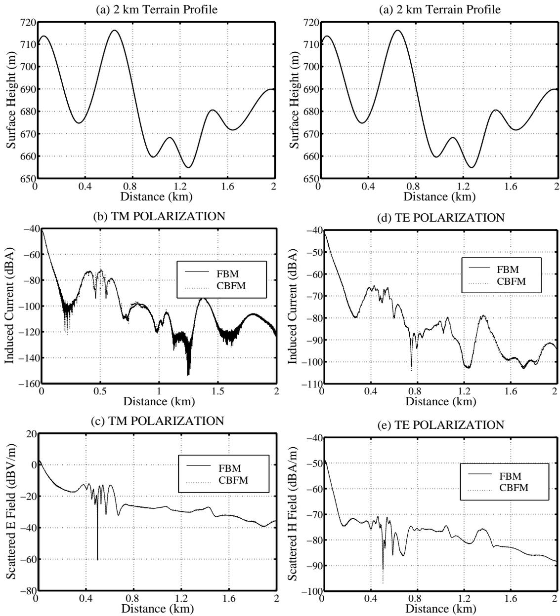
Figure 1. Scattering from a  $2000\lambda$  Terrain Profile.
