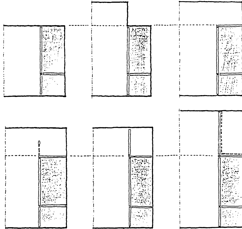
Fig 6 : Partial sections of various solutions for the bedding closets in traditional rooms. (Source: Küçükerman, 1989).
