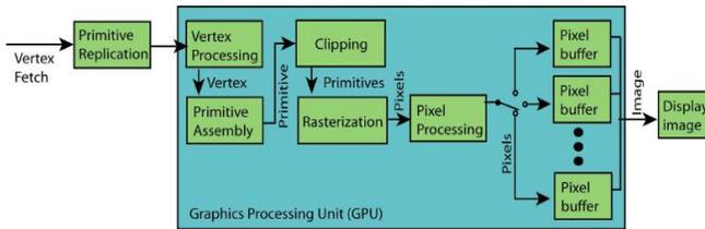
Figure 2: The modified rendering pipeline for Stereoscopic
