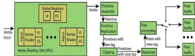
**Figure 1:** The Unified Rendering pipeline for multi-view autostereoscopic rendering. Here VI and VS refer to viewpoint-independent and viewpoint-specific registers respectively.
