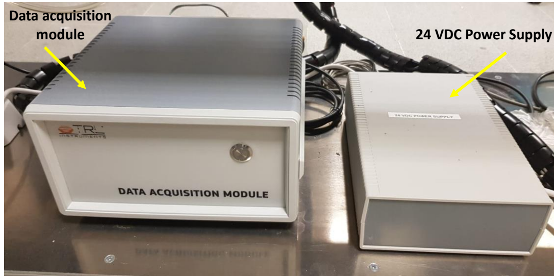
Figure 2-11. Data acquisition module and 24 VDC power supply.
