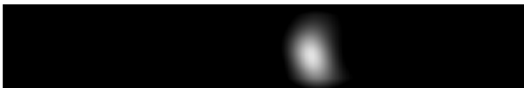
Figure 5.5: First projection image of a point source phantom acquired with the scanner. Imaged phantom consists of a 5 times diluted Perimag sample that is contained inside a 2-mm wide capillary tube. Full width half max dimensions of the acquired image of phantom is 3 mm along the z-direction and 5 mm along the x-direction.
