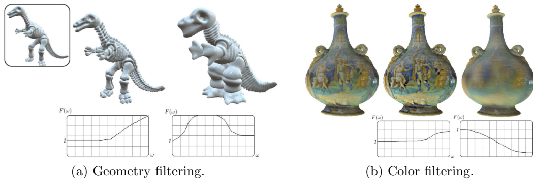
Figure 3.7: Filtering different attributes of a mesh with MHT (Image from [101], courtesy of Bruno Levy, reprinted with permission).
