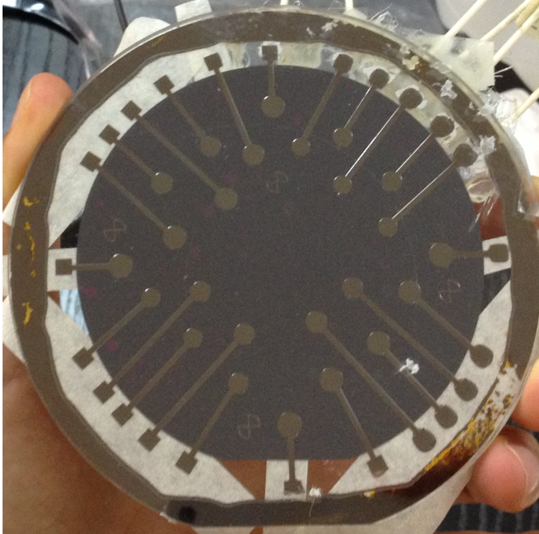
Figure 4.2: Front view of fabricated CMUT wafer that have 24 CMUT cells.
