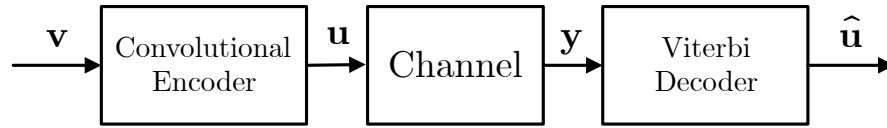
Figure 2.12: Flowchart of the convolutional coding with Viterbi decoding.
