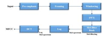
Fig. 1. Block Diagram of MFCC
