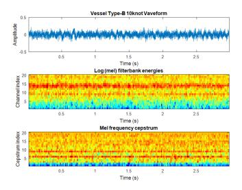
Fig. 9. Type-B 10knot filterbank energy and MFCC
