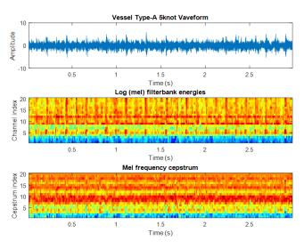
Fig. 7. Type-A 5knot filterbank energy and MFCC
