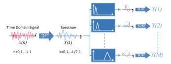
Fig. 3. Mel-Filter Bank Processing
