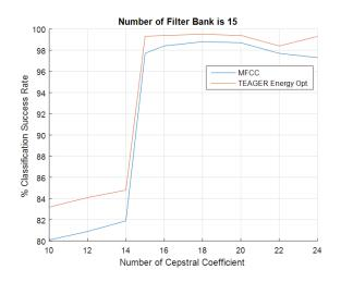
Fig. 11. Performance of methods according to # of Cepstral Coefficients
