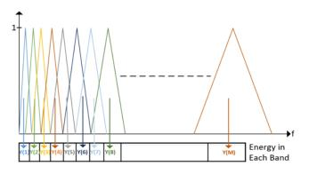
Fig. 2. Triangular Mel-Scale filter bank
