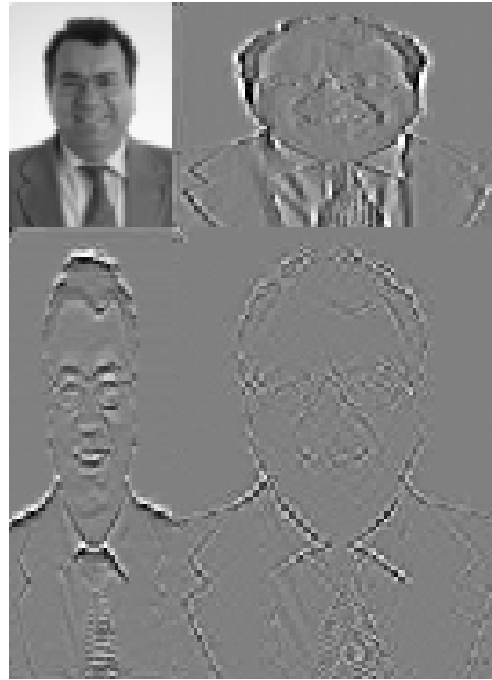
Figure 8. 2D unbalanced lifting wavelet transformed image with p=3:1 and q=3:2 . Highband subimages are amplified by a factor of three.
