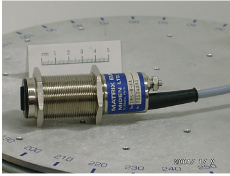
Figure 1. A closeup view of the infrared sensor.
