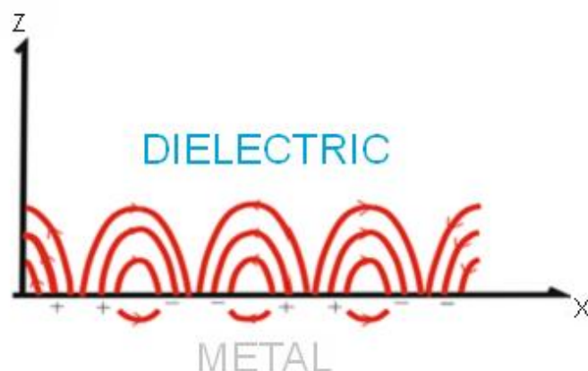
Figure 2.1: Surface Plasmons between metal, dielectric media
