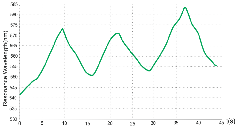
Figure 6.2 : \pm 0,4 V applied voltage; silver as plasmon supporting metallic layer and 0,05 M CuSO4 solution as dielectric media
