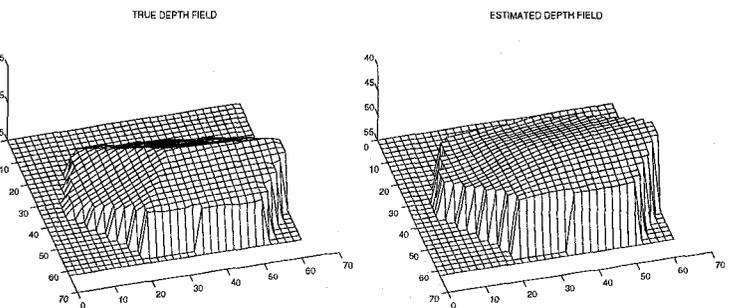
Figure 3: The mesh representations of the true and encoded depth field of the current frame of the "Cube" sequence.
