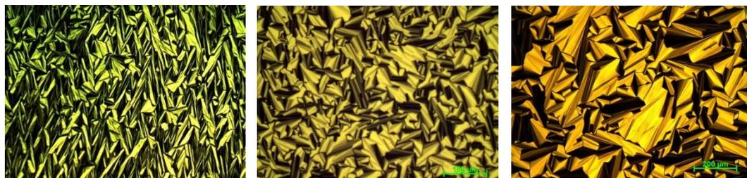
**Figure 4.31.** The POM images of  $2.0\text{LiI}-0.2\text{I}_2-x\text{H}_2\text{O}-\text{C}_{12}\text{EO}_{10}$ ,  $2.0\text{LiI}-0.5\text{LiCl}-0.2\text{I}_2-x\text{H}_2\text{O}-\text{C}_{12}\text{EO}_{10}$ , and  $2.0\text{LiI}-0.5\text{LiBr}-0.2\text{I}_2-x\text{H}_2\text{O}-\text{C}_{12}\text{EO}_{10}$  samples from left to right.
