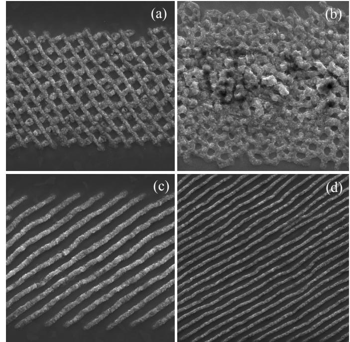
Fig. 4. SEM images of titanium dioxide nanopatterns formed on titanium surface: (a) mesh-wire structure created by double-pass with 90°-rotated polarization, (b) nanocircles created by circularly polarized light, (c) double-pass with same polarization, showing the permanence of the structures, (d) structure showing that lines from multiple, partially overlapping passes can be stitched to form a structure of arbitrarily large area.
