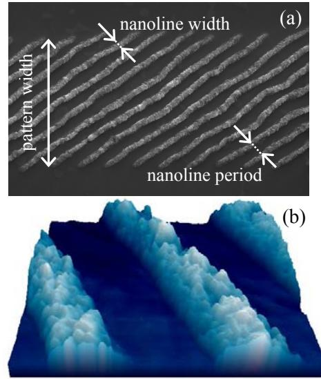
Fig. 2. (a) SEM and (b)  $2 \times 2 \mu\text{m}^2$  AFM images of nanolines formed with at 95 mW of incident average power.
