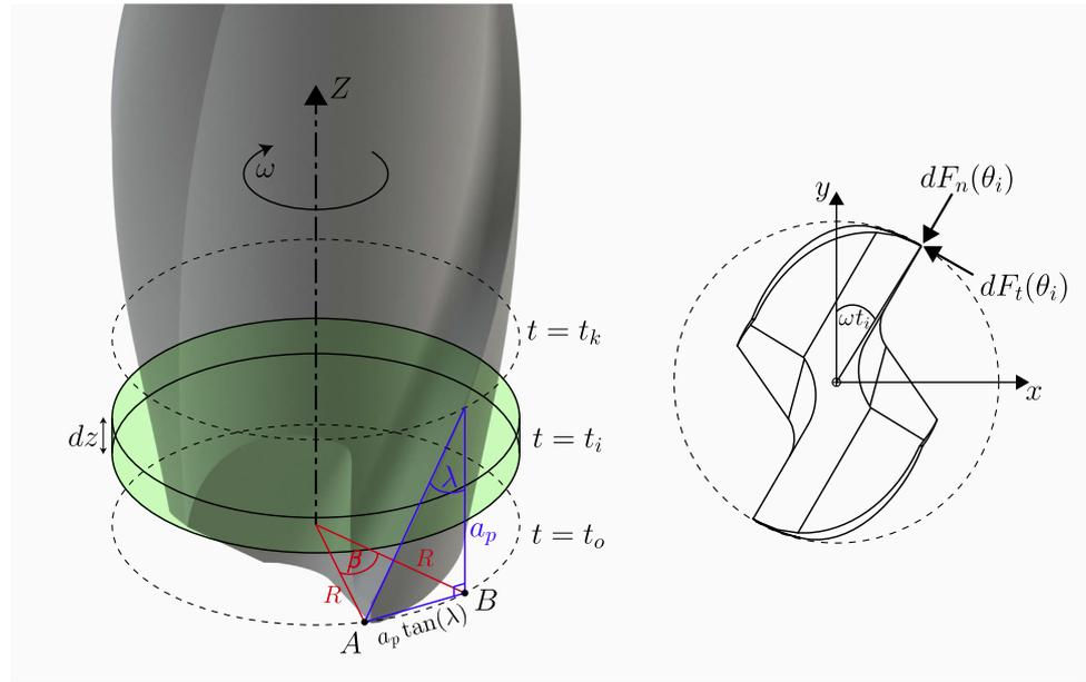
The cutting forces in the tool reference plane are calculated using Eq. 5 and then transformed into the reference plane of the workpiece using Eq. 7:
