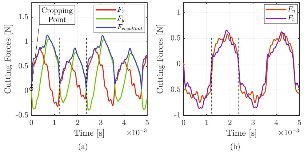
**Fig. 18** Splitting and averaging the force signal. (a) Tangential force. (b) Normal force
