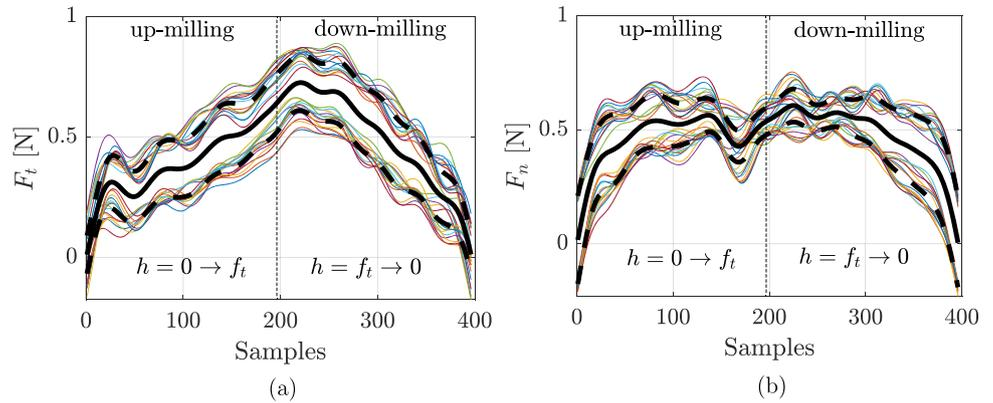
**Fig. 19** Curve fitting the force signal. (a) Tangential force. (b) Normal force
