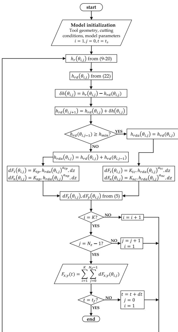
Fig. 9 Flow chart of the force model
