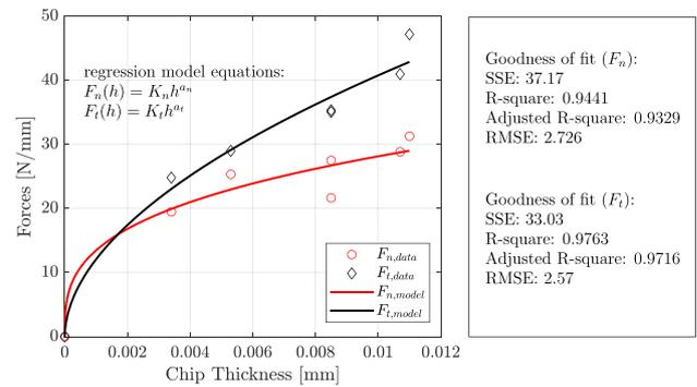
Fig. 20 Curve fitting of the chip/force data pairs and identification of the cutting coefficients
