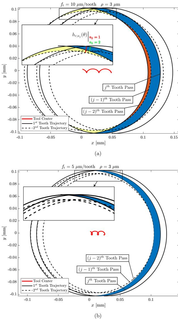
**Fig. 4** Simulated cutting tooth trajectories in two different cases: (a)  $f_t = 10 \mu\text{m/tooth}$ ,  $\rho = 3 \mu\text{m}$ . (b)  $f_t = 5 \mu\text{m/tooth}$ ,  $\rho = 3 \mu\text{m}$
