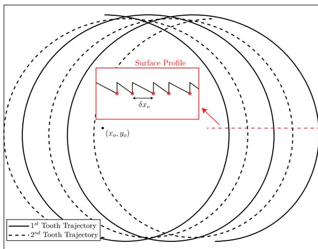
**Fig. 6** Influence of tool runout and deflection on the centerline surface topography
