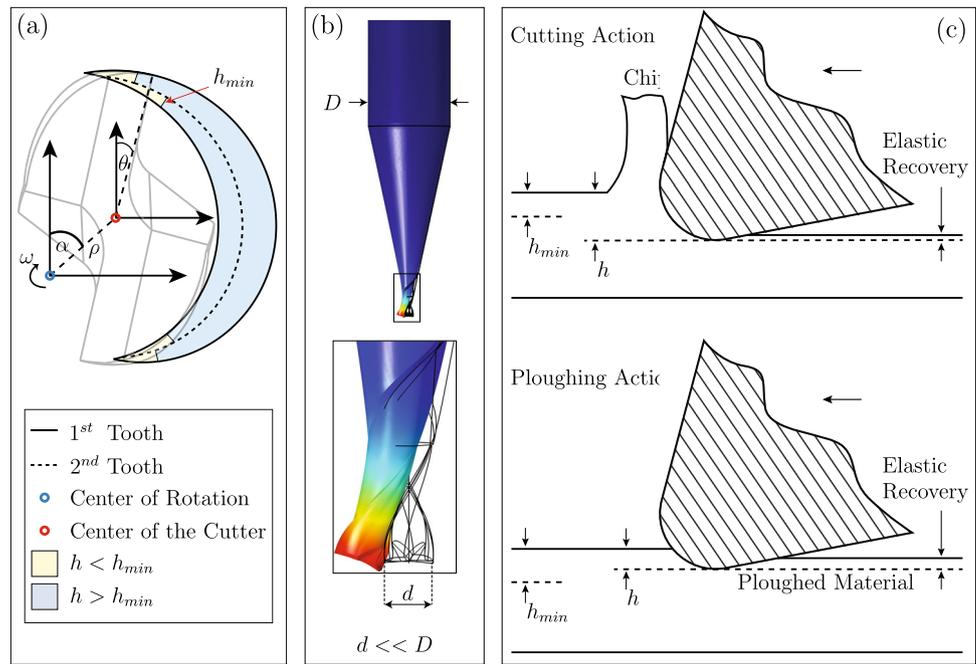
and the helix lag. An initial value of the uncut chip thickness assuming a rigid tool is calculated from the trochoidal trajectory of the teeth considering runout. Tool deflection (Fig. 1b) through a finite element based model and chip thickness accumulation due to ploughing action (Fig. 1c) are also considered in the model. The details of the model are explained below.
