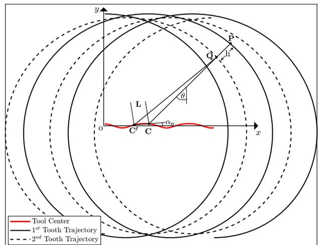
**Fig. 3** Simulated trajectory of the cutting teeth of a two-flute ( $N_z = 2$ ) micro-end-mill
