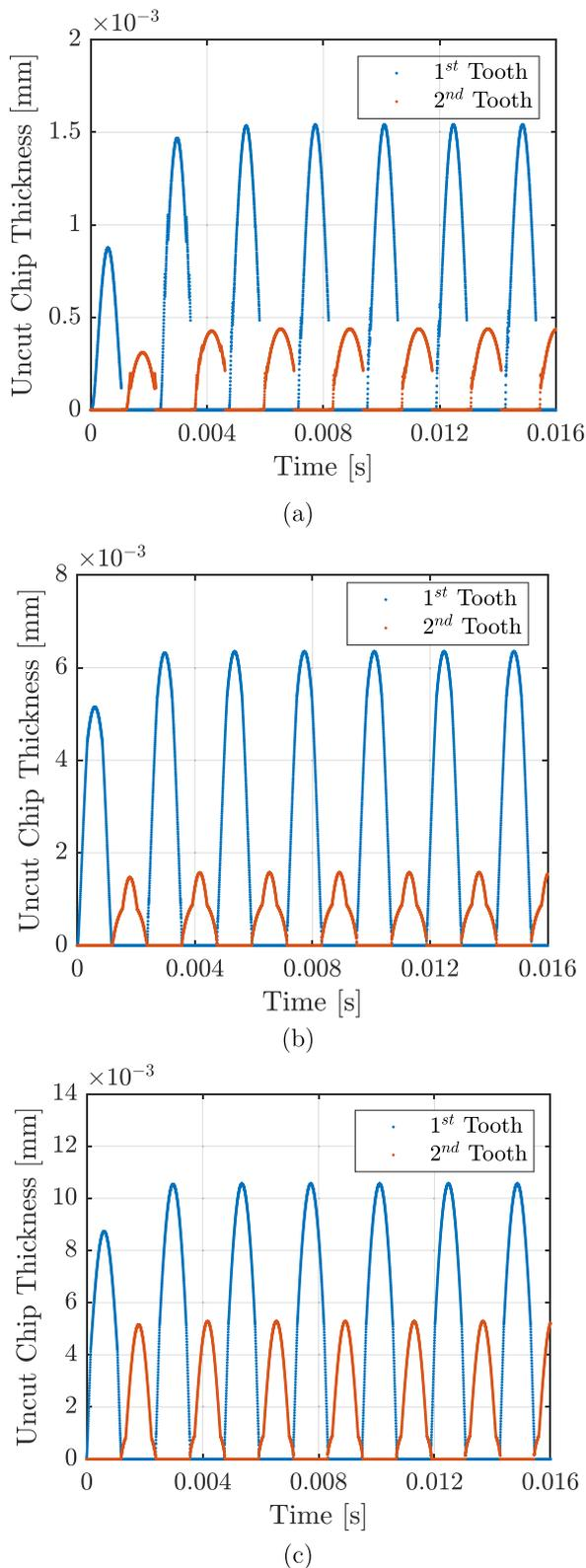
**Fig. 21** Simulated uncut chip thickness at (a) 1  $\mu\text{m}/\text{tooth}$ , (b) 4  $\mu\text{m}/\text{tooth}$ , and (c) 8  $\mu\text{m}/\text{tooth}$
