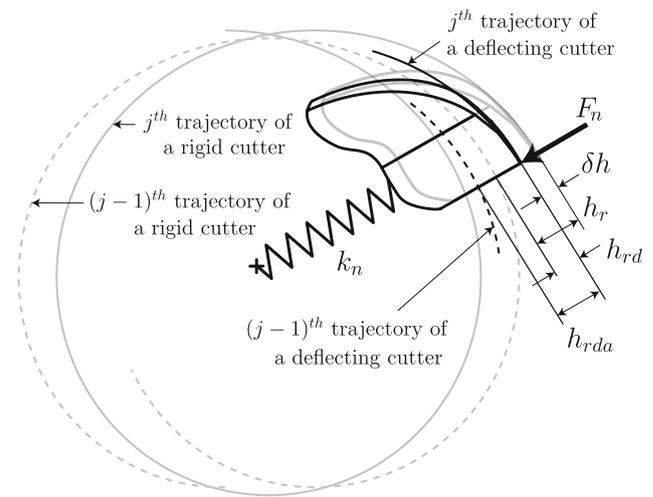
**Fig. 5** Illustration of the influence of micro-end-mill deflection on the chip thickness
