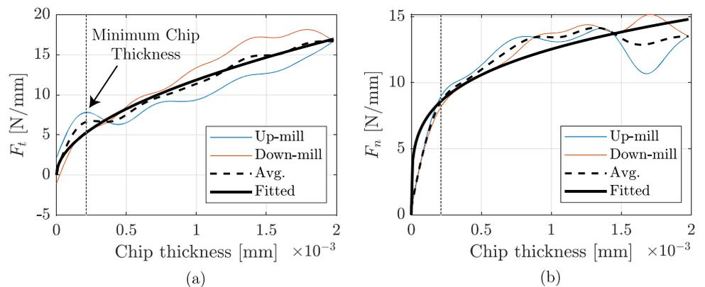
tests were conducted using the same tool and workpiece, while keeping the spindle speed constant at 25000 rpm, the feed constant at 4 μm, and varying the axial and radial depth of cut as shown in Table 1. The cutting length of the tests was 2 mm. The side wall surfaces were scanned with the laser scanning microscope using a 50× objective lens, and horizontal profile measurements were taken at three different heights at 25-μm increments on the side walls.
