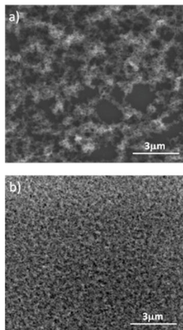
Figure 1: SEM images of ormosil thin films prepared by using gels synthesized in different solvents (a) methanol, (b) DMSO.
