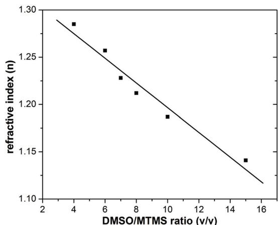
Figure 2: Refractive index change of the ormosil coatings with changing monomer concentration.
