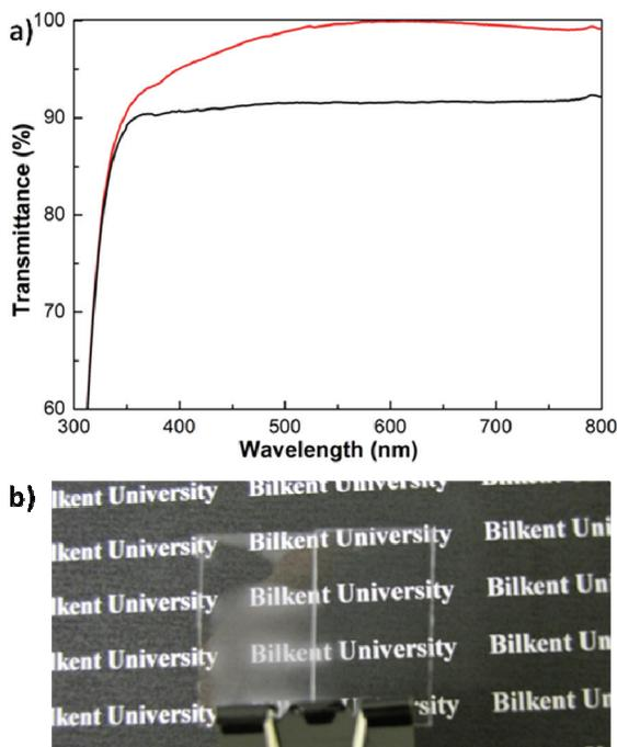
Figure 5: (a) Transmission spectra of glass substrate (black) and ormosil coated glass substrate (red) (b) Photograph showing the antifogging property of annealed ormosil coating on glass.
