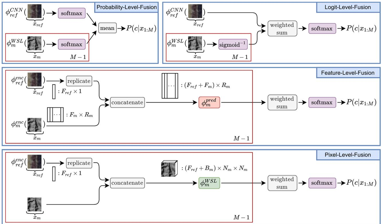
Fig. 4. Illustration of the proposed multisource WSL models. The reference source  $x_1$  is represented with subscript  $ref$ , while subscript  $m \in \{2 \dots M\}$  is used for the additional sources. Plate notation is used to represent the repetitions in the model. Variables are described in the text.
