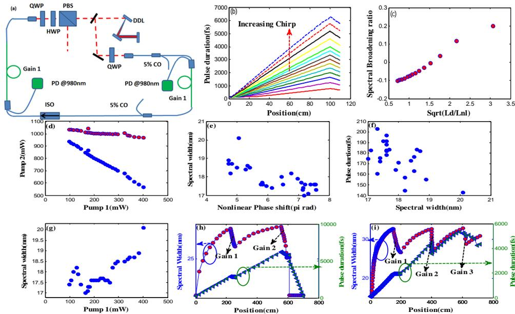
**Fig. 1** (a) Schematic of the laser. (b), (c) Two-segment simulation showing the effect of chirp on spectral compression in Yb-gain fiber. Experiment (d-g) showing relationship between, (d). Two PP. and TP (Red) in the cavity. NLPS with (e). SW, (f). CPD, (g). SW with PP1. Simulation(h and i) (h). Dynamics of double gain oscillator and, (i). Dynamics of a cascade of gain and passive fiber.
