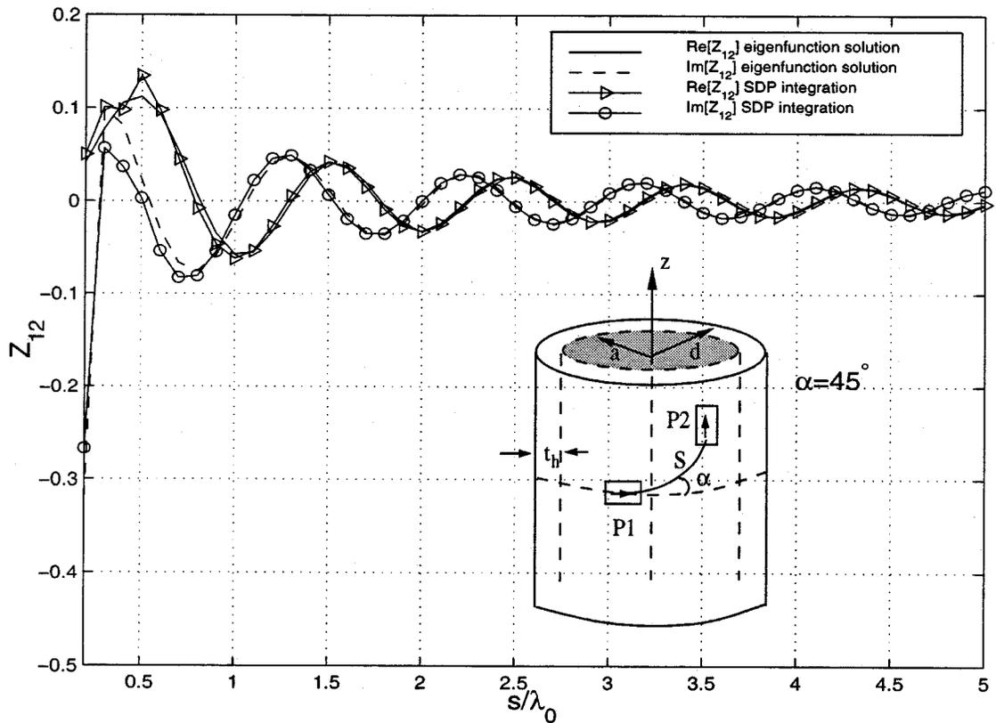
Fig. 6. Real and imaginary parts of the mutual impedance between  $z$ - and  $\phi$ -directed current sources for a coated cylinder with  $a = 3\lambda_0$ ,  $t_h = 0.06\lambda_0$ ,  $\epsilon_r = 3.25$ .
