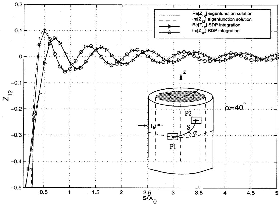
Fig. 7. Real and imaginary parts of the mutual impedance between two identical  $\phi$ -directed current sources for a coated cylinder with  $a = 3\lambda_0$ ,  $t_h = 0.06\lambda_0$ ,  $\epsilon_r = 3.25$ .
