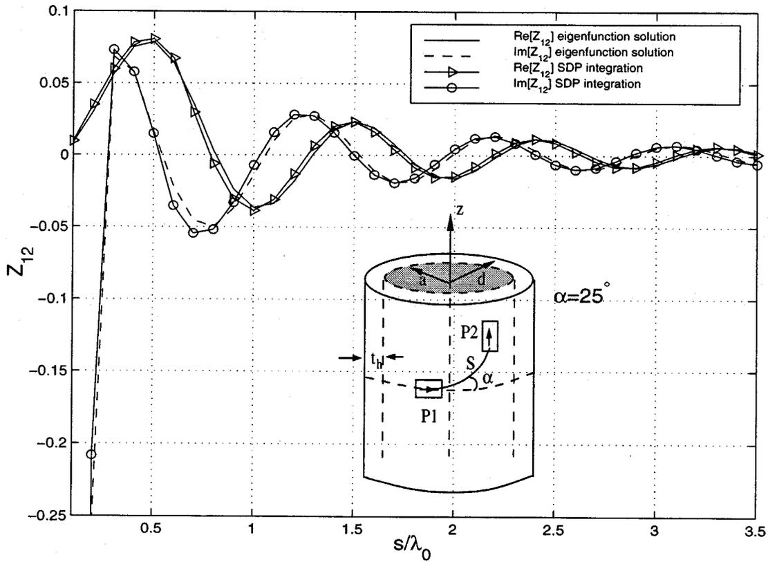
Fig. 9. Real and imaginary parts of the mutual impedance between  $z$ - and  $\phi$ -directed current sources for a coated cylinder with  $a = 1.5\lambda_0$ ,  $t_h = 0.06\lambda_0$ ,  $\epsilon_r = 3.25$ .
