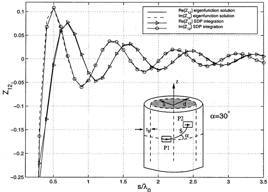
Fig. 10. Real and imaginary parts of the mutual impedance between two identical  $\phi$ -directed current sources for a coated cylinder with  $a = 1.5\lambda_0$ ,  $t_h = 0.06\lambda_0$ ,  $\epsilon_r = 3.25$ .
