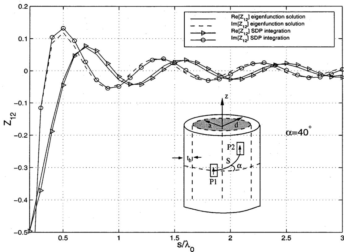
Fig. 8. Real and imaginary parts of the mutual impedance between two identical  $z$ -directed current sources for a coated cylinder with  $a = 1.5\lambda_0$ ,  $t_h = 0.06\lambda_0$ ,  $\epsilon_r = 3.25$ .
