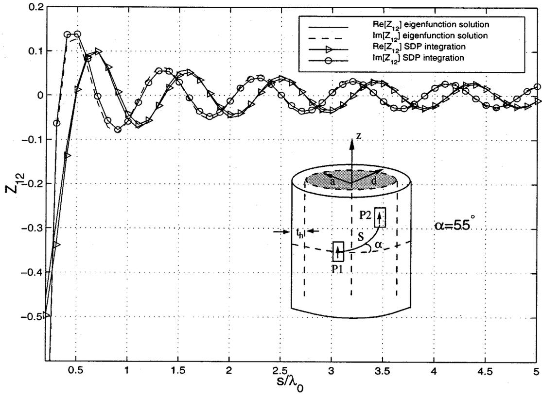
Fig. 5. Real and imaginary parts of the mutual impedance between two identical  $z$ -directed current sources for a coated cylinder with  $a = 3\lambda_0$ ,  $t_h = 0.06\lambda_0$ ,  $\epsilon_r = 3.25$ .  $Z_{12} = \int \mathbf{E}^{(1)} \cdot \mathbf{J}^{(2)} d_3$ , where  $\mathbf{J}^{(2)}$  is source  $P_2$  and  $\mathbf{E}^{(1)}$  is the field due to source  $P_1$ .
