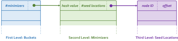
Figure 6: Memory layout of the hash-table-based index.
