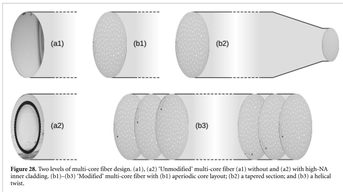
modification post-drawing of the multi-core fiber tip—a tapering or a homothetic transverse downscaling over a few centimeters (figure 28(b2))—can dramatically increase the PSF intensity while introducing virtually no additional energy exchange and leaving the memory effect intact [196].
