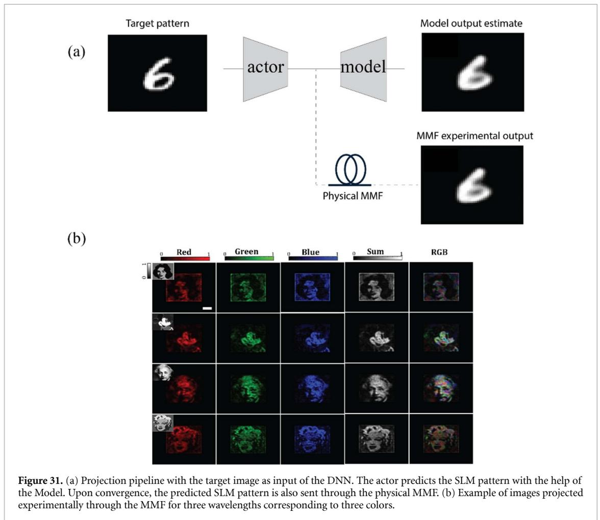
**Figure 31.** (a) Projection pipeline with the target image as input of the DNN. The actor predicts the SLM pattern with the help of the Model. Upon convergence, the predicted SLM pattern is also sent through the physical MMF. (b) Example of images projected experimentally through the MMF for three wavelengths corresponding to three colors.
