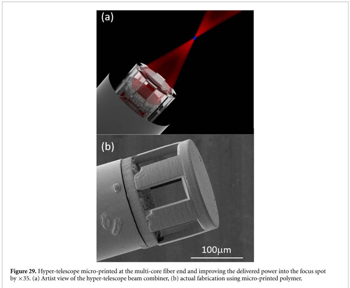
**Figure 29.** Hyper-telescope micro-printed at the multi-core fiber end and improving the delivered power into the focus spot by  $\times 35$ . (a) Artist view of the hyper-telescope beam combiner, (b) actual fabrication using micro-printed polymer.
