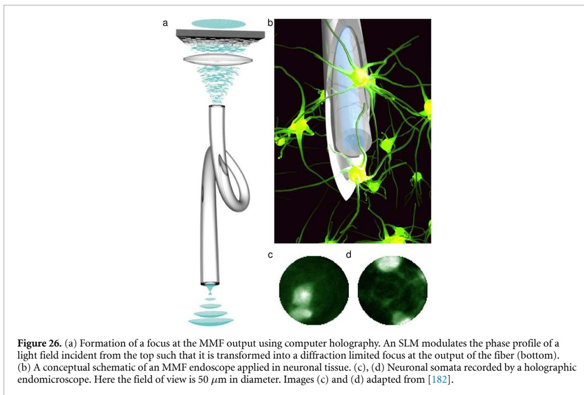
**Figure 26.** (a) Formation of a focus at the MMF output using computer holography. An SLM modulates the phase profile of a light field incident from the top such that it is transformed into a diffraction limited focus at the output of the fiber (bottom). (b) A conceptual schematic of an MMF endoscope applied in neuronal tissue. (c), (d) Neuronal somata recorded by a holographic endomicroscope. Here the field of view is  $50\ \mu\text{m}$  in diameter. Images (c) and (d) adapted from [182].
