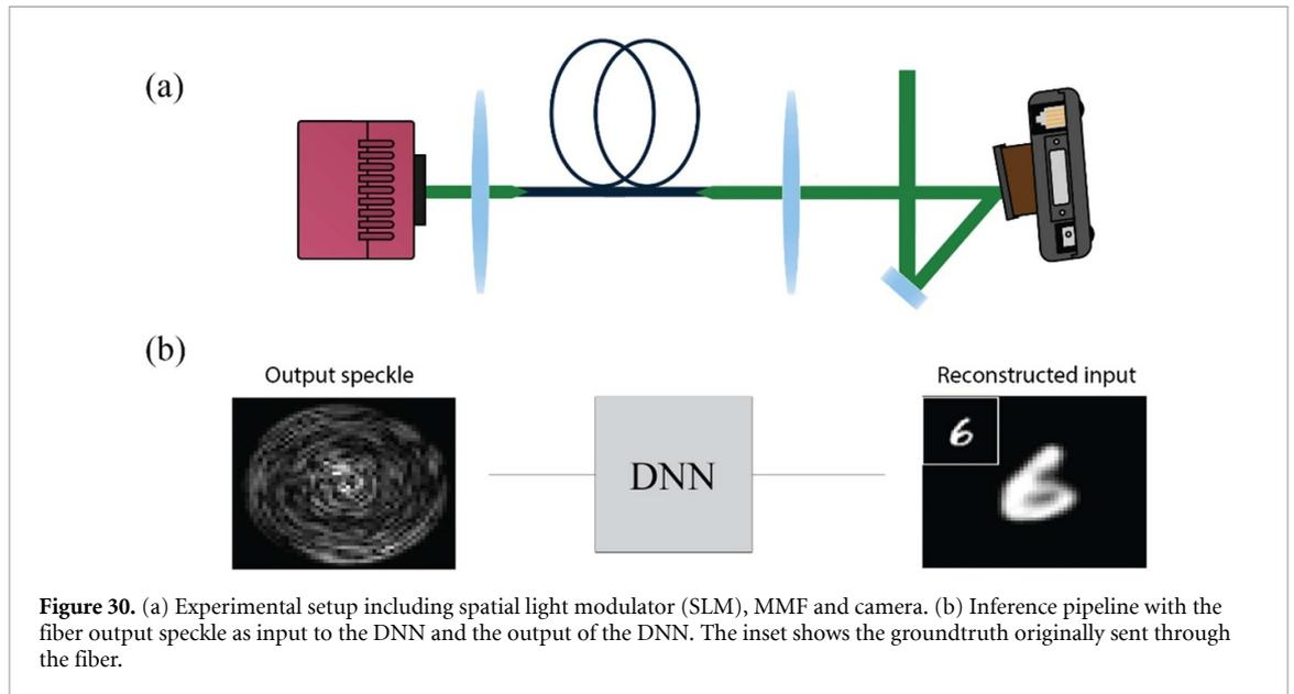
**Figure 30.** (a) Experimental setup including spatial light modulator (SLM), MMF and camera. (b) Inference pipeline with the fiber output speckle as input to the DNN and the output of the DNN. The inset shows the groundtruth originally sent through the fiber.
