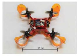
Fig. 1. Miniature, foldable, collision resilient quadcopter, MiniCoRe.
