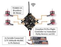
Fig. 7. Setup of the finalized electronic suite equipped with Crazybee F4 Pro.
