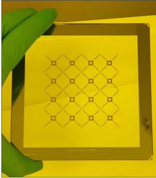
Figure 2.58: The image of produced and planned to use Silicon Etch mask.
