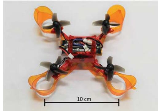
Fig. 1. Miniature, foldable, collision resilient quadcopter, MiniCoRe.
