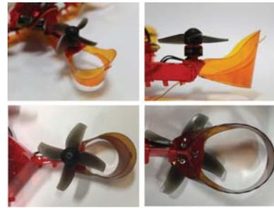
Fig. 6. Implementation of the bumper, mounting point and half-fold is visible.
