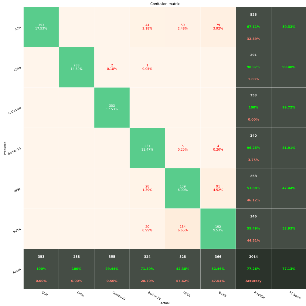
Figure 4.9: Confusion matrix of the WVTFI technique for test data of 6 class set at 0 dB SNR level.
