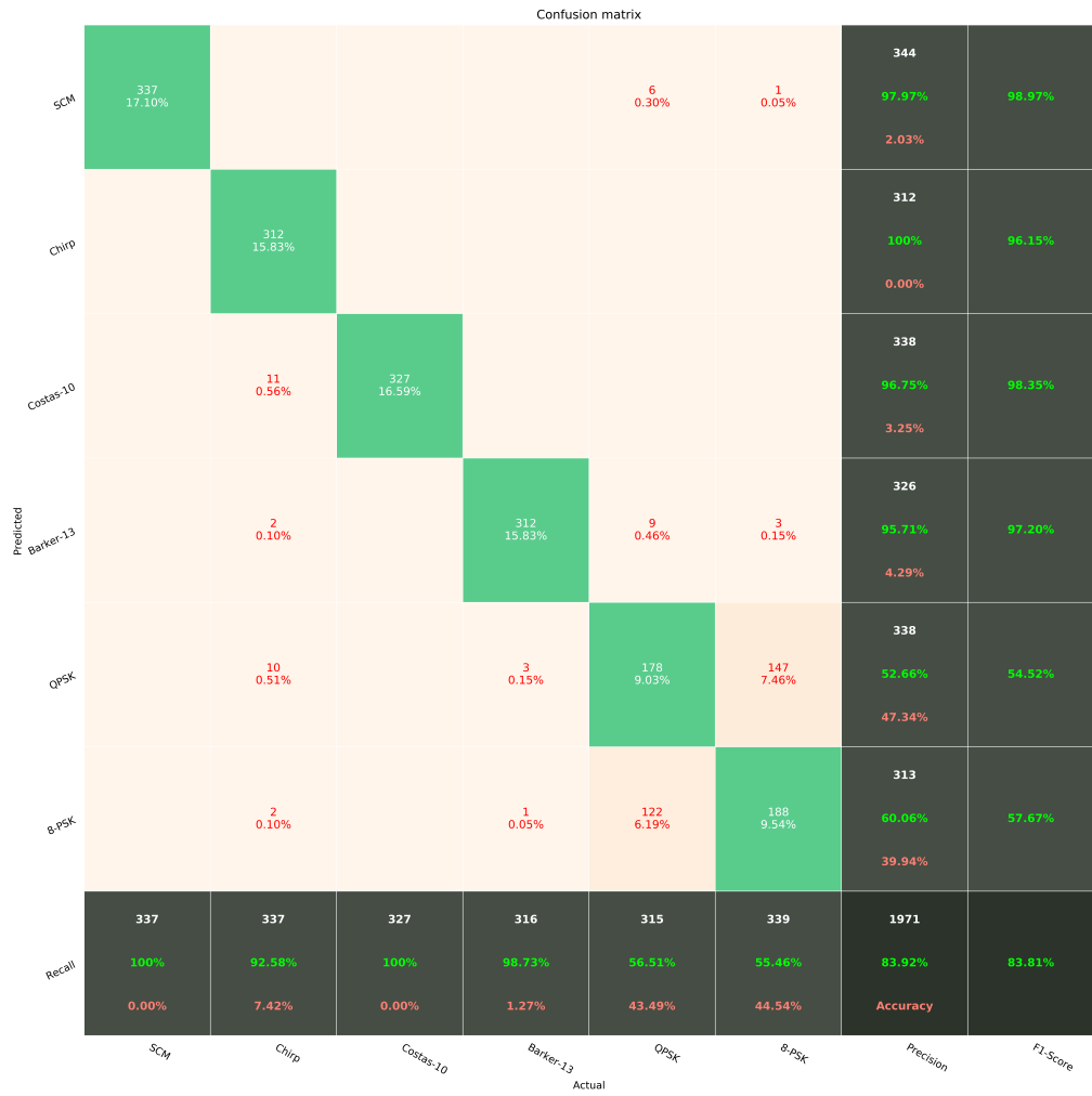
Figure 4.7: Confusion matrix of the pure CNN based model for test data of 6 class set at -10 dB SNR level.
