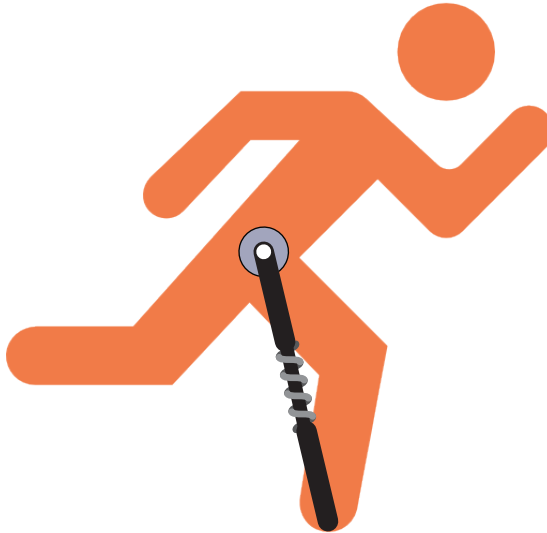
Figure 1.1: Representation of Running with Spring Loaded Inverted Pendulum [1,2]
