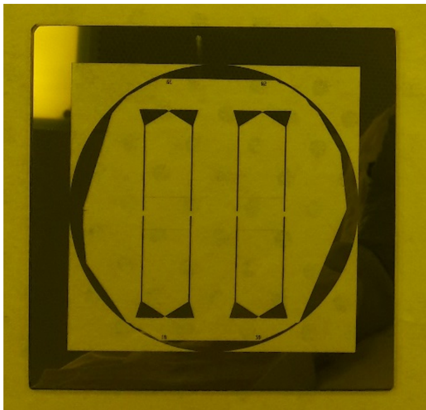
Figure A.1: Photolithography mask used for cell detection & flow rate sensor
