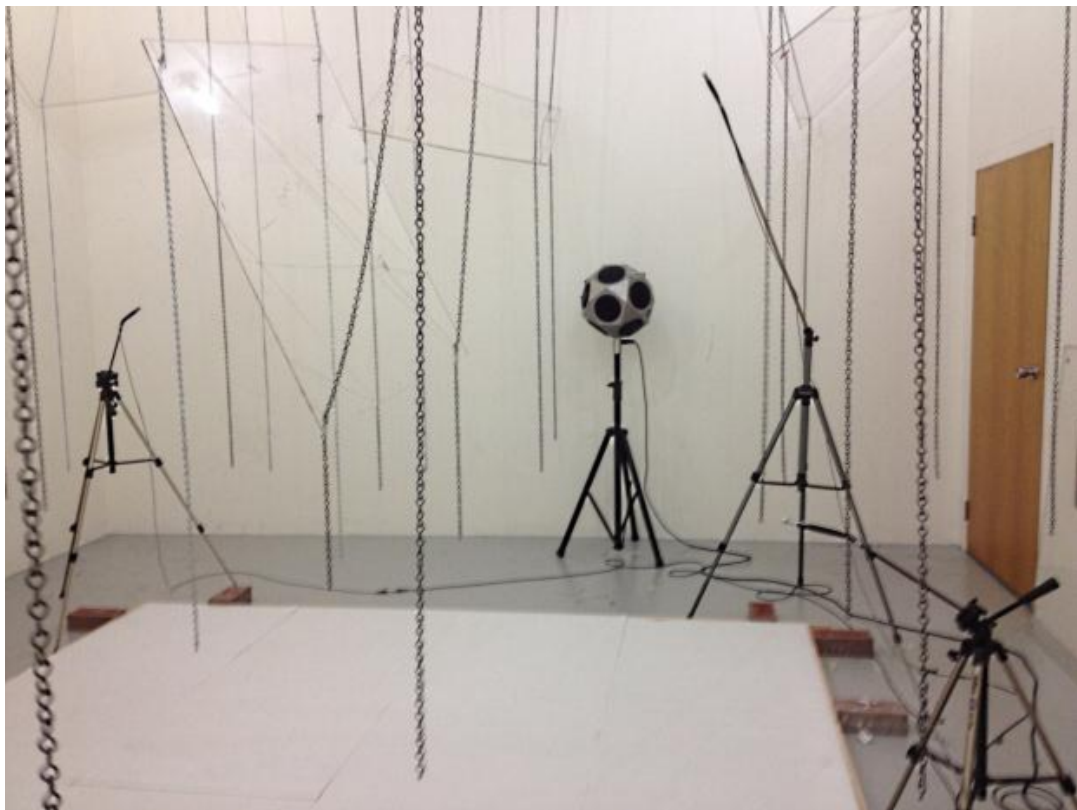
Figure 2.4: A photograph showing reverberation room measurement set-up [4].
