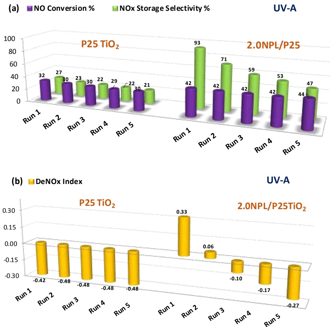
Figure 3.30: Long term %NO conversion, %NO x storage selectivity and DeNO x index results of P25 and 2.0NPL/P25 under UV-A light irradiation.
