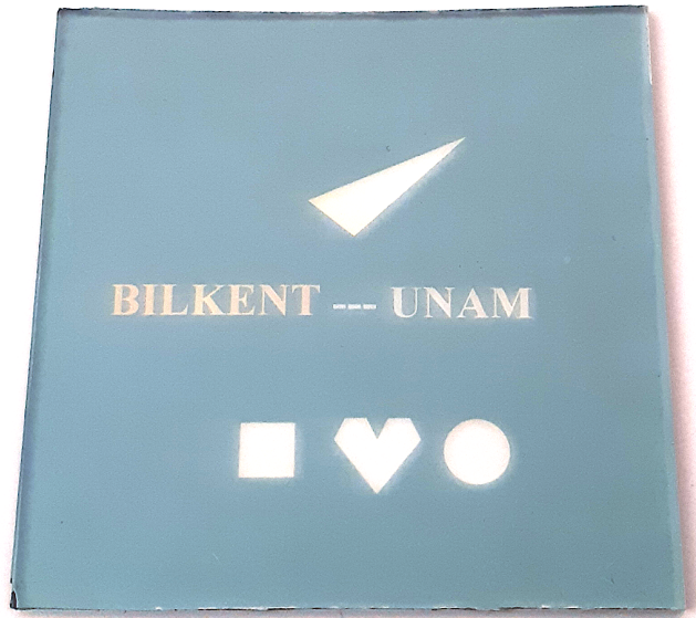
Figure 4.1: Coated glass sample. The writings and the shapes were drawn by ablating the coating with different laser parameters.
