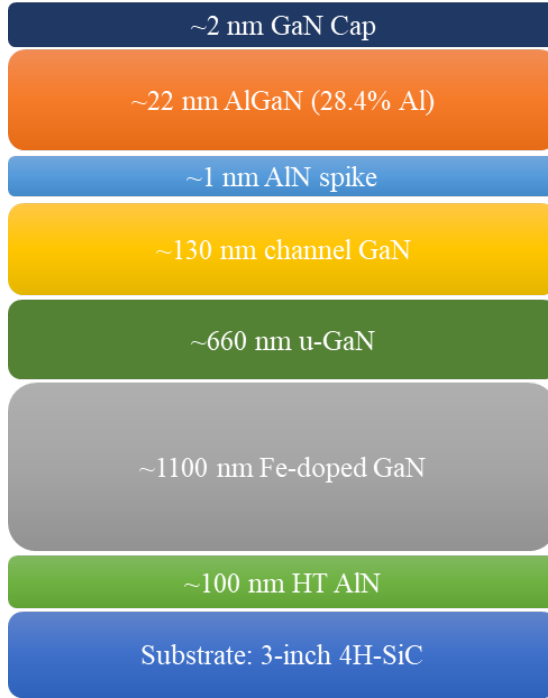
Figure 2.1: Epitaxial structure showing the layers grown by MOCVD.
