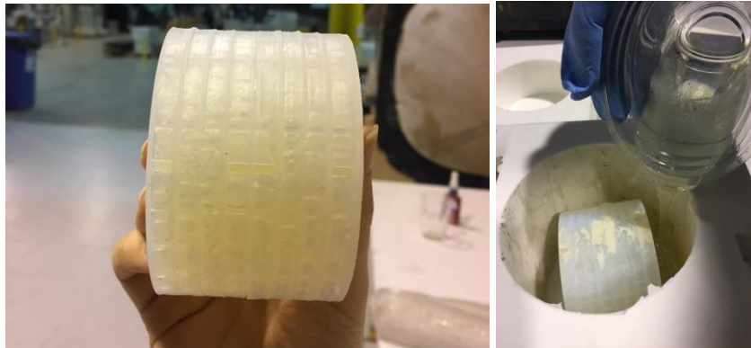
Fig. 4 Final printout of Web Labyrinth (WL) sample in real size (on the left), while epoxy resin is being cast to the mould to have the final version suitable for Kundt tube measurements. (on the right)
