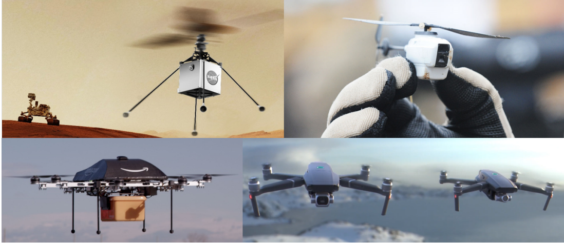
Figure 1.2: Examples of drones and their practical utilities. NASA 2020 Mars Scout (top left) is a contra-rotating helicopter robot, DJI Mavic Zoom & Mavic 2 (top right) aerial photography drones, Prox Dynamics AS Black Hornet Nano MAV used for military reconnaissance purposes (bottom left), Amazon Prime Air delivery drone (bottom right).
