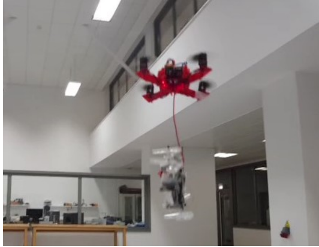
Figure 5.5: Fol-Quad air-lifting another foldable robot Vasler (35 grams).
