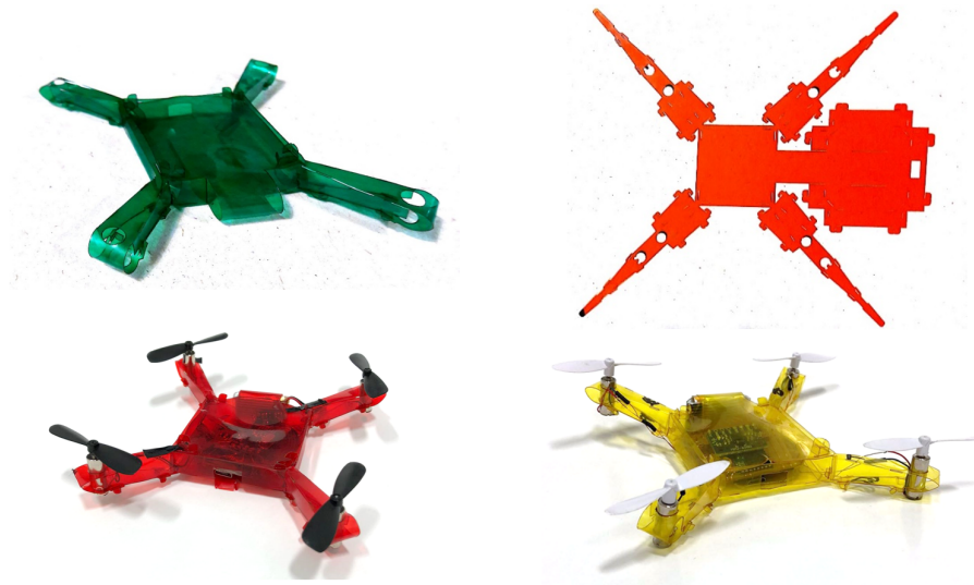
Figure 3.3: First prototype of the foldable micro quadrotor equipped with Arduino Nano, MPU6050 IMU, and coreless DC motors.
