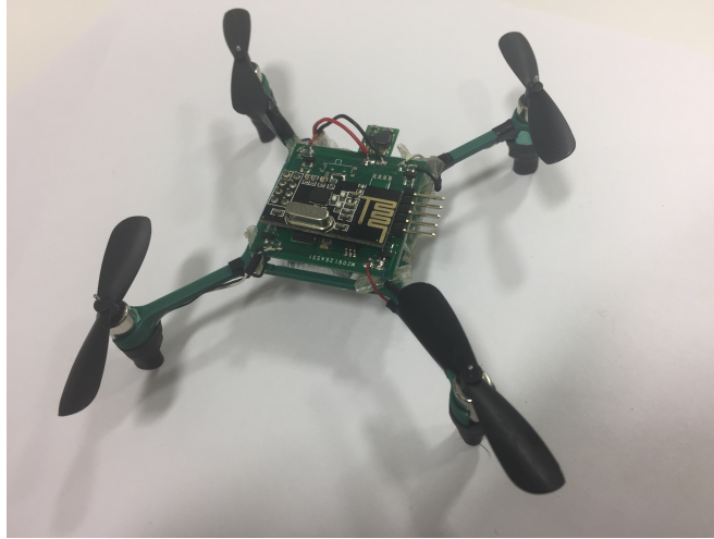
Figure 5.3: 3D printed frame quadrotor with PMFC, coreless motors and final version of the PCB.
