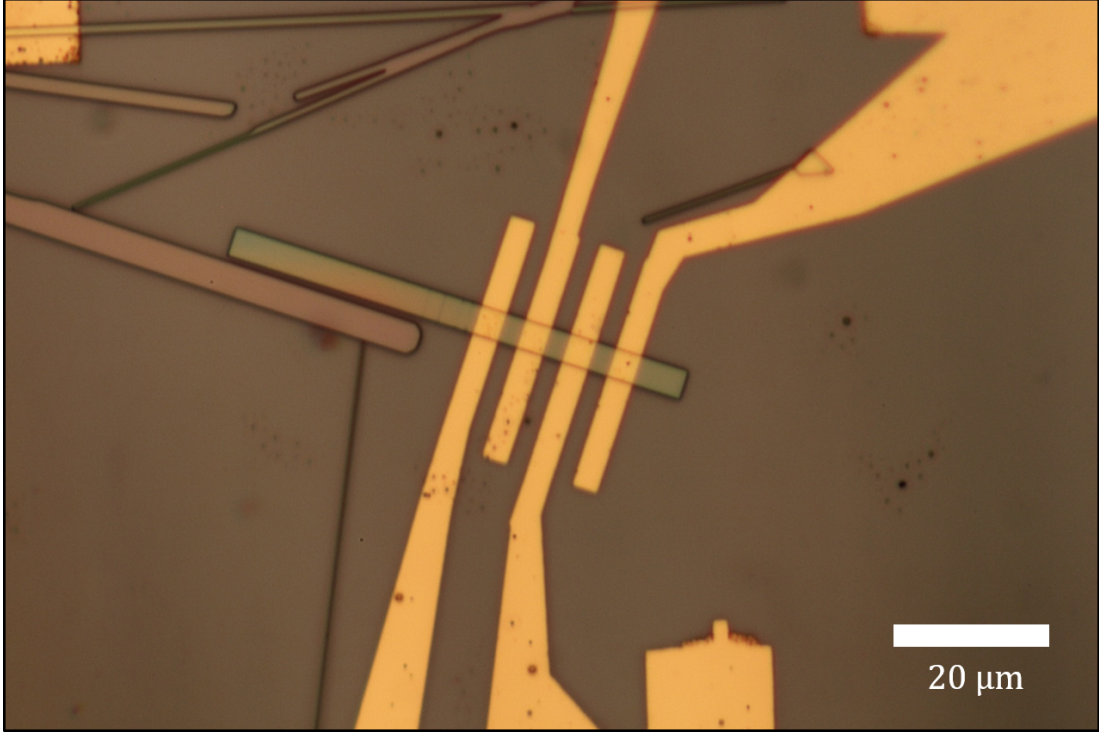
Figure 3.11: Optical image of a 4-terminal VO 2 device used in magnetoresistance measurements.
